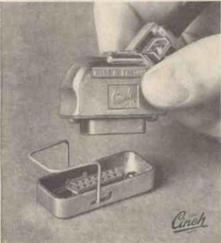
These connectors consist of one-piece Diallyl Phthalate moulding with hard gold plated plug pins, socket contacts, and beryllium copper contact clips. Closed entry contact design eliminates the risk of damage to the sockets by test probes. The shells are of passivated cadmium plated steel and the covers and cable clamps are of die-cast aluminium Grade LM6.
