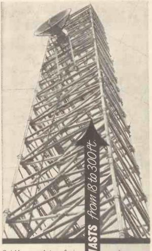
Quickly erected (300 ft. in 6 hours) for temporary links, emergency communication, outside broadcasts and survey. Interchangeable one-piece folding tower sections fit one on top of the other and include enclosed stairway with platforms, ensuring safety at heights even for the inexperienced. Each section weighs only 100 lbs. No elaborate base required. Air transport-Weatherproof-all aluminium - and thoroughly tested in the field. In regular use, in snow and sun, in all continents.
