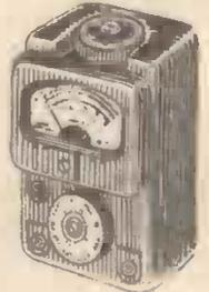
A must for the home constructor. Sensitivity: 1,000 ohms per volt. A.C. and D.C. Ranges (A.C./D.C.): 0-10-50-250-500-1,000 v. D.C. current 0-100-500 m/a. (used at 0-10 v. range.) Resistance 1-2,000 ohms (centre 24 ohms), 100-200,000 ohms (centre 2.4 k.). Size 5 x 3 x 2½in. Complete with test leads.
