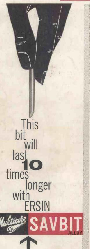
Developed after prolonged research in the Multicore Laboratories, Ersin Multicore Savbit Type 1 Alloy lengthens the life of copper soldering iron bits by up to ten times. It incorporates a small percentage of copper, and this prevents absorption of copper from the bit into the solder alloy. By keeping the bits in good condition, the use of Ersin Multicore Savbit Alloy speeds soldering and increases efficiency.
