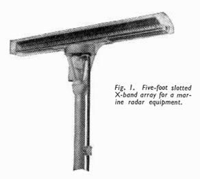
data on the performance of the aerial, and has the great advantage that these tests can be carried out in the laboratory. Having obtained the desired characteristics, the polar diagram measurements need only be carried out as a final check. This method was used for the development of the X-band slotted array shown in Fig. 1.
