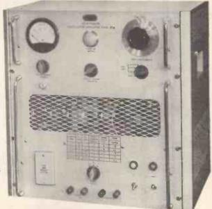
The High Power Oscillator/Amplifier is an instrument which combines an L.F. oscillator operating over the frequency range 30 c/s to 30 kc/s with a power amplifier capable of delivering up to 150 watts into a wide range of output impedances. The amplifier output is monitored by means of a built-in Voltmeter and an input socket is provided for use with external signal sources (microphones, pick-ups,
