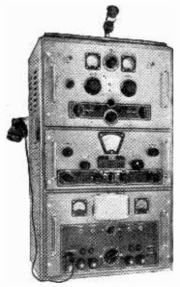
Radio Becker marine R/T transmitter and receiver Type HB-3/75-DSK. The transmitter (135W) operates on 33 channels between 17 Mc/s and 1,600 kc/s, and the receiver has a built-in auto alarm.
