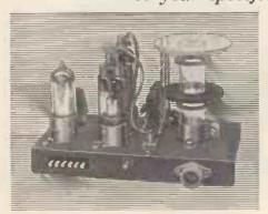
Compact Stabilised High Voltage Supply. Safe and reliable supply for photo-multiplier cells and cathode ray tubes. Variable output between 0-1250V D.C. at 250 micro amps. Size 6"×4"×3".
