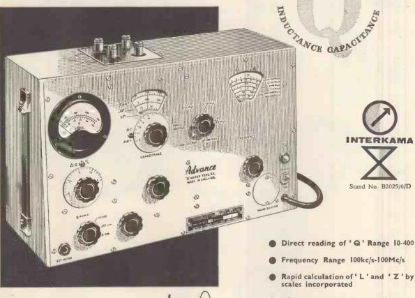
The 'Q' Meter Model T2 is a reliable instrument for making measurements of circuit magnification, inductance, capacitance and power factor at frequencies between 100 kc/s and 100 Mc/s. The variable-capacitor control has three calibrated scales which greatly simplify the calculations of inductance and impedance. A comparison facility is incorporated to enable batch testing by unskilled personnel.
