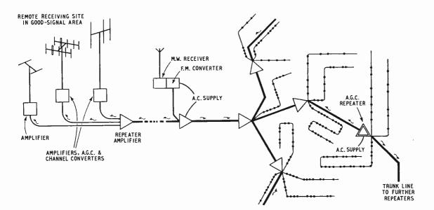
Fig. 7. Layout of hypothetical Band I/f.m. distribution system. Heavy lines represent trunk cables feeding further repeaters. Typically 40 to 60 subscribers can be fed from one line.
