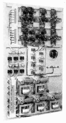
Fig. 6. Belling-Lee main-station equipment. At top are module aerial amplifiers and converter. Band I and f.m. repeater amplifier in centre with space for Band-III wideband amplifier. Separate power units for each section aid reliability. Equipment is on swing-out door of cabinet.
