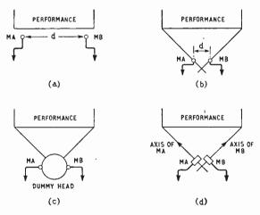
Fig. 19. Microphone arrangements. (a) Widely spaced omnidirectional microphones. (b) Closely spaced omnidirectional microphones. (c) Omnidirectional microphones mounted in artificial head. (d) Closely spaced directional microphones.
