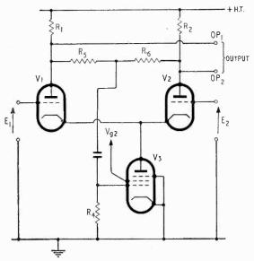
Fig. 3. Long-tailed pair with feedback.
