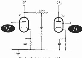
Fig. 1. Basic push-pull amplifier.
