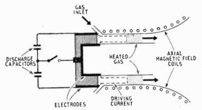
Fig. 2 Schematic of one proposed type of plasma shock propulsion motor. (Based on Fig. 7 of an article by M. Camac, A. Kantrowitz and H. E. Petschek in the April 1959 issue of "I.R.E. Transactions on Military Electronics.")
