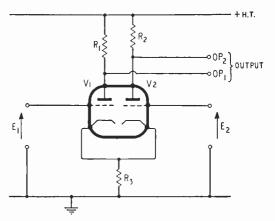
required h.t. line. Provided that a constant anode voltage is maintained, the gain of the amplifier, which may typically be one hundred times, is independent of the value of  $R_3$ . However, in practice, the above ideal conditions could not be realized for any length of time because of valves and component ageing. This is where the common cathode resistance  $R_3$  becomes useful.
