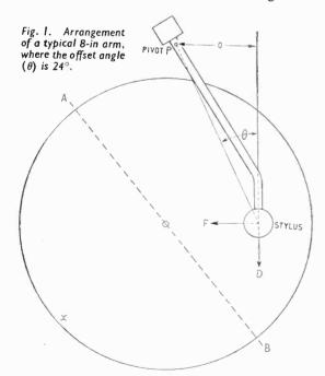
the record groove at the point of contact. This is in the direction D on the diagram, and its line of action is displaced from the pivot (P) to the extent of the linear offset (O). Thus this forward force produces a clockwise moment about the pivot which tends to press the stylus against the inner groove wall in the direction F.
