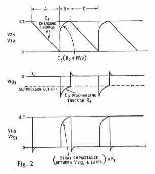
h.t.  $C_2$ , now discharging towards zero volts, reaches the V1 suppressor grid cut-off point and anode current begins to flow again in V1. This causes the voltage at V1 anode and V2 grid to fall. The current in V2 starts to fall and the voltages at V2 anode and V1 suppressor rise. This cumulative action
