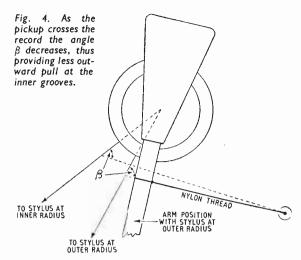
This is useful as a rough guide to the weight needed at a given distance from the pivot or to the distance from the pivot needed for a given weight.
