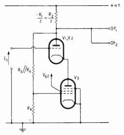
Fig. 7. Circuit of Fig. 3 simplified for push-push operation.
