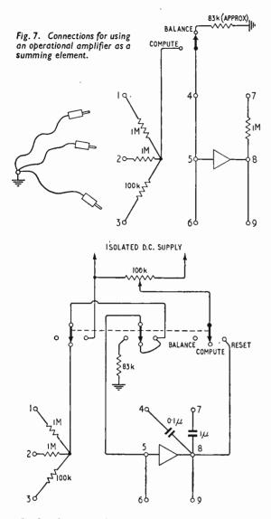
Fig. 8. Connections for using an operational amplifier as a summing integrator.
