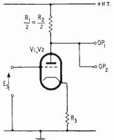
push-push signal. In Fig. 2, if R<sub>1</sub> is equal to R<sub>2</sub> and V1 and V2 are identical, then once again the pushpush rejection will be infinite. However, if R<sub>1</sub> is not equal to R<sub>2</sub> there will be a component of the interference signal in the output voltage between terminals OP<sub>1</sub> and OP<sub>2</sub>.
