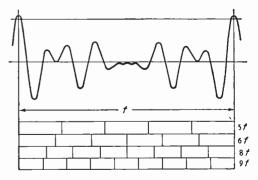
Fig. 2. The combination of all four frequencies sent out by each station in turn generates this lane identification pulse at the receiver. The main peaks, at f, create a coarse navigational pattern to reduce ambiguity.
