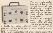
This extremely useful, low priced device will extend the use of your single-beam oscillo-scope for duties otherwise only in the pro-vince of the double-beam tube.
