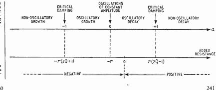
If we take a practical case, for instance a tuned circuit having a Q of 50 and resonating at 1 Mc/s when the capacitance is 150 pF, the resistance required for deadbeat growth of current has to be more negative than (-2000) ohms.
