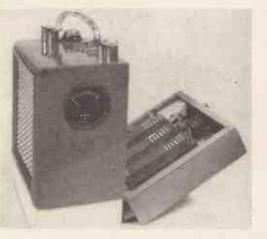
230 c/s, and the air volume in the box after the insertion of components was 26 cu in, which brought the peak up to 390 c/s. Allowing for losses in an attenuator and in the components which correct for variations of loudspeaker impedance with frequency, a maximum power of  $\frac{1}{4}$  W is needed from the transistor circuit.
