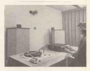
Over 50% of the production time of Beam-Echo (Avantic) equipment is devoted to testing. The photograph shows the final llstening test on an SPA21 stereophonic combined pre-amplifier and  $2 \times 12$ -watt amplifier being performed in a near acoustically dead room.
