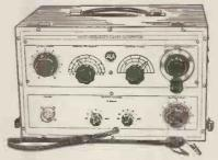
Laboratory type equipment designed for alignment of wide band RP and IF amplifiers. Comprises generator and regulated power supply unit each housed in grey crackled steel case 17 × 10 × 12in. Centre Frequency 5-56 Mois. Sweep width 0.2-20 Mois. Marker oscillator frequency 5-70 Mois. Operates from 105-125/210-230 v. A.C. Mains. Complete with 13 valves and Technical handbook. BRAND NEW condition. £39/10/-. Carr 10/-
