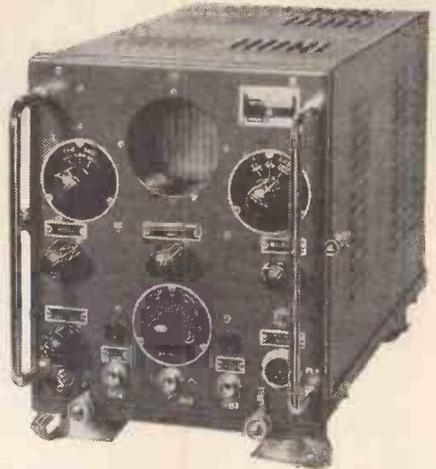
**MARCONI SIGNAL GENERATORS TF-517-F/1.** Special offer of these Laboratory Signal Generators. Cover 10-18 Mc/s, 33-58 Mc/s, and 150-300 Mc/s. In good, used condition, with charts. Checked before despatch. Complete with power pack for normal A.C. mains. **ONLY £12/10/-** (carriage, etc., 20/-).
