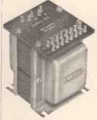
30-WATT TYPE Ref. WO866 Primary inductance > 250 H. Leakageinductance < 4 in H. Wide Frequency range at full power. H.F. response level to >80K~. 7,000/3.7/15 ohms, 43% pri. taps for E.L. 34's, KT66's or 807's.
