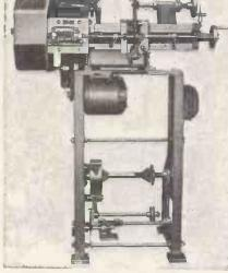
DIAMETER OF COIL 10" . LENGTH OF COIL 12" WIRE GAUGES 10 TO 30 S.W.G. PRICE 6150
