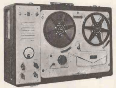
The amplifier, speaker and case, with detachable lid, measures  $8\frac{1}{4}$  in. x  $22\frac{1}{2}$  in. x  $15\frac{3}{4}$  in. and weighs 30 lb.
