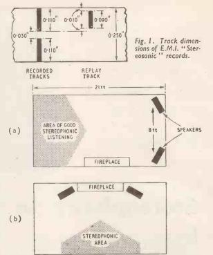
Fig. 2. Alternative positions tried for the loudspeakers in a living room.
