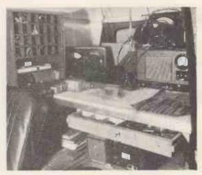
ON-THE-SPOT fitting of car radio within the Greater London area is now provided by Rootes Ltd., who have equipped a van specially for the task. It is a combined installationdemonstration vehicle and is itself fitted with the new 20X Radiomobile receiver. Being on call (Ladbroke 3232) it obviates motor traders carrying stocks of radio parts.
