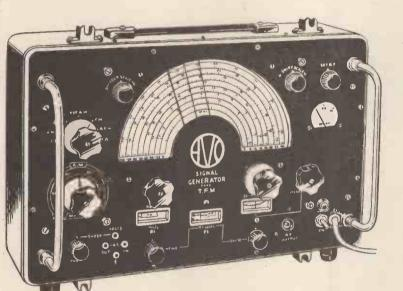
A M COVERAGE 5-220 Mc/s in 8 ranges, CW or 400 c/s sine/square wave modulation. Accuracy ± 1%. Provision for spot frequency calibration.
