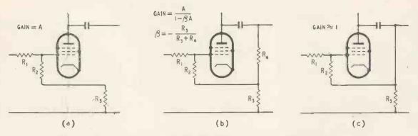
Fig. 5. Equivalent circuits of Fig. 4 at (a) low, (b) mid-band, and (c) high frequencies.
