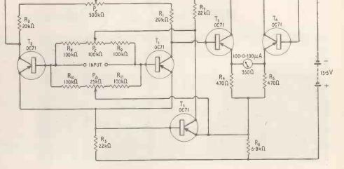
Fig. 6. Final circuit with additional compensation for the effect of temperature on the zero setting.
