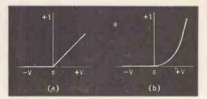
Fig. 2. Transistor demodulation characteristics: (a) an ideal curve giving linear demcdulation; (b) the actual characteristic with demodulation and gain non-linear.
