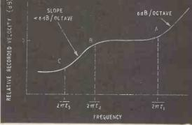
Fig. 2. General form of standard recording characteristic.
