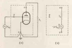
Fig. 2. (a) The essentials (so far as a.c. is concerned) of the most familiar basic type of valve circuit, in which the input (a signal source) is connected between g and k, and the output (a load resistance) between a and k. (b) The valve equivalent.
