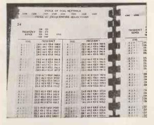
Specimen of calibration table as it appears after the film record has been registered with the printed frequency table.
