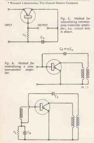
Fig. 7. Method similar to that shown in Fig. 6, but with r, and C, taken into account.
