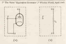
Fig: 1. (a) represents an actual valve, with its grid signal voltage relative to cathode kept at zero by short-circuiting g to k. (b) is the equivalent circuit of the valve under these conditions; it can be substituted for (a) for purposes of a.c. signal calculations.
