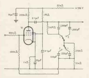
Fig. 6. Complete equalizer for B.S.S. 1928 : 1955 characteristics. VI may be Z729, EF86, 6BR7, etc. Mid-band gain approx. 10. Switch positions: 1—B.S.S. Coarse Groove, 2—B.S.S. Fine Groove.
