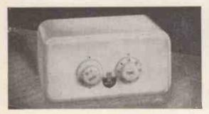
The Wolsey Convertor Is a self-contained unit complete with power pack, comprising transformer with tapped primary for mains voltage selection, together with metal rectifier and R.C. smoothing.
