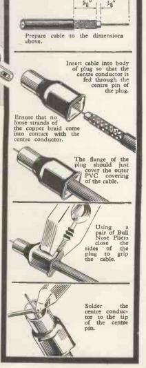
The illustrations above show the extremely simple and speedy method of fitting the plug.
