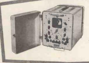
For distortion measurements on working circuits without interrupting service. Each element of a start-stop signal appears separately on the spiral time base display. Adjustable speeds from 20-80 bauds. Weight 33 lb. Higher speed versions can be supplied to order.
