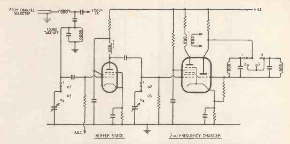
Fig. 4. Use of a second frequency changer for sound, giving a second i.f. of either 11.8 or 7 Mc/s. The buffer stage is switched between 27.75 and 33.4 Mc/s. (Switch positions: 4, France; 2, Belgium and Luxembourg; 3, Belgium and Luxembourg; 4, C.C.I.R.)
