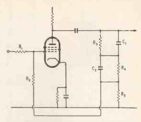
Fig. 4. Equalizer employing negative feedback. The resistor  $R_{\delta}$  (shown dotted) is normally omitted, but may be included, if necessary to limit the low-frequency boost.
