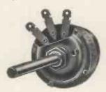
STANDARD CARBON POTENTIO-METERS. Made by an entirely new method ensuring a highly stable resistance element, which is also very durable. Silent and smooth in operation, these controls offer both mechanical and electrical reliability. Soldering tags are heavily silver plated to resist oxidisation, and the mains switch has an efficient quick make-and-break action.
