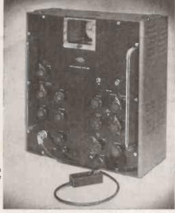
THE OSCILLOSCOPE TYPE 830 has been designed for general wide-band frequency work and is particularly suitable for observing pulse waveforms with very fast rise-times. The frequency response of the Y amplifier is flat from 30 c/s to 20 Mc/s and the time-base provides writing speeds up to 20 cms. per microsecond.
