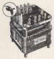
Optimum conditions are obtained in the form of output stage used in this amplifier when about 40% of the primary winding of the output transformer is common to anode and screen grid circuits. The Partridge Type P.3878 is of C-core design with tappings of 43% of primary turns, and is specified by the designer for this amplifier.
