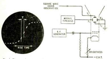
Fig. 1. Time markers derived from the positive half-cycles of a radio-frequency input to the c.r.t. grid.
