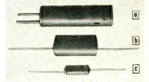
Steps in the miniaturization of capacitors. All units are  $2 \mu F$  and (a) is paper and metal foil construction, (b) is metallized paper and (c) is the new metallized lacquer film type. The largest capacitor is  $2\frac{1}{2}$  in long.
