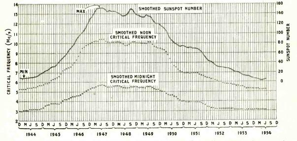
Fig. 1. Twelve-month running average of sunspot numbers and of noon and midnight F2 critical frequencies over the sunspot cycle.
