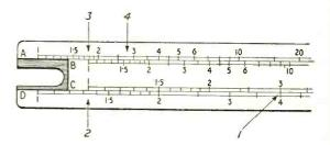
Fig. 1. The first steps in setting the slide rule are shown here, culminating in  $1 + (x,y)^2$  at point 4.
