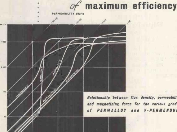
Relationship between flux density, permeability and magnetizing force for the various grades PERMALLOY and V-PERMENDUR.
