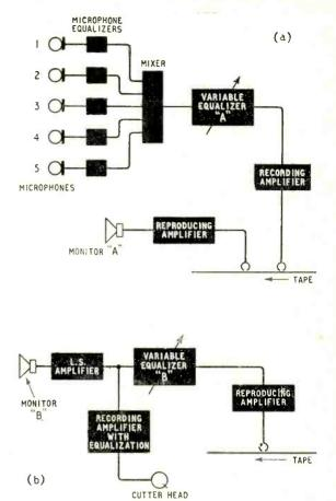
Fig. 2 Stages in the production of a lacquer "cut"; (a) recording the tape master, (b) transcribing from tape to disc.
