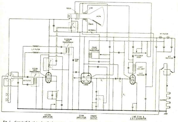
Fig. 1. Circuit of 3-valve subscriber's receiver. The eight contacts of the input plug on the left carry the following: 1 and 2, vision and scanning signals on carriers; 3 and 4, sound at speech-coil level; 5 and 6, mains supply; 7, brightness control voltage: 8, earth connection.
