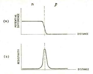
Fig. 15. Graph showing resistivity in different parts of the crystal.
