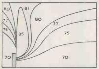
Fig. 1 Diagram showing the heat zones produced by a typical 1 kW natural convection heater. The upwards and outwards path of the warm air is quite clearly indicated. If the power of the heater were increased to 2 kW, temperatures in the particular zones would increase, but the general disposition of the zones would remain the same. The air at floor level would thereforebe noticeably colder. (Temperatures in both illustrations are in degrees Fahrenheit.)
