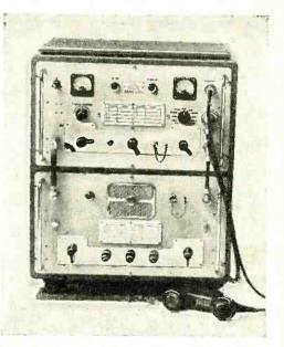
oscillator is also crystal-controlled, and in addition to covering the same frequency range as the transmitter the set provides for reception on 200 kc/s (Droitwich). The combined set measures 24m high  $\times$  20in wide  $\times$  10in deep.
