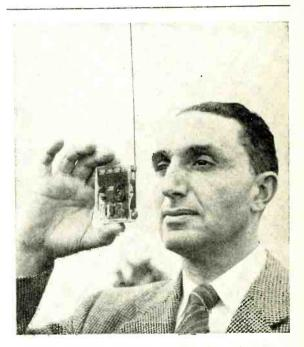
ONE way of solving the battery problem—but perhaps more suitable for nomadic Arabs than for stay-al-home Britons is exemplified by this new transistor transmitter, which is powered entirely by sunlight through the medium of selenium cells. Built by Edward Keonjian (General Electric Company of America), it has a range of about 100ft.
