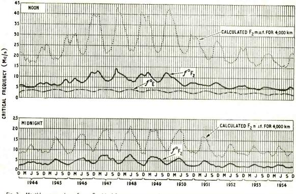
Fig. 2. Monthly mean values of noon E critical frequency, noon and midnight  $F_2$  critical frequencies, and noon and midnight  $F_2$  m.u.f.s over the sunspot cycle.
