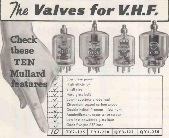
Ten features to bear in mind—plus the assurance that these valves are already being widely employed with marked success in both communications and industry. The triodes TY2-125 (CV1924) and TY3-250 are recommended for grounded-grid R.F. amplifiers in communications equipment and as oscillators in compact R.F. heaters. The tetrodes QY3-125 (CV2130) and QY4-250 (CV2131)—included in the Services Preferred Types List—are characterized by high power gain and high efficiencies at V.H.F.
