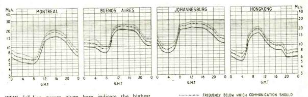
THE full-line curves given here indicate the highest frequencies likely to be usable at any time of the day or night for reliable communications over four long-distance paths from this country during February.
