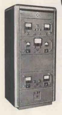
Abbreviated Specification Frequency range 60-216 mc/s Transmitter output Power Io watts, or with Amplifier Unit-50 watts Maximum Deviation 50 kc/s Overall Transmitter-Receiver Performance Frequency Response 300 c/s-6 kc/s±3 db 6 kc/s-36 kc/s±1 db Intermodulation Level At least-55 dbm for 2 tones applied each at 0 dbm Receiver Bandwidth 6 db down + 120 kc/s
