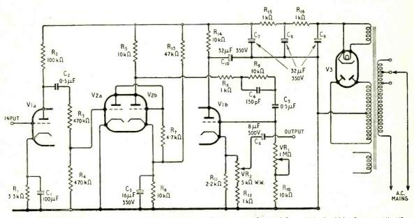
Fig. 1. Circuit diagram of square-wave shaper. All resistors 1-watt except  $R_{15}$  and  $R_{16}$  which should be 5-watt. VI, V2, ECC33 or ECC82; V3, GZ30 or EZ80.
