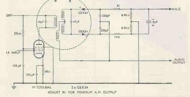
Transformer Design. Although the circuit shown above is conventional, an I.F. transformer designed for use with thermionic diodes is not necessarily the most suitable for germanium diodes. A suitable design of transformer has been evolved at The G.E.C. Research Laboratories, details of which are available on request.
