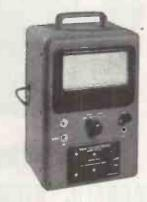
All-purpose test set enabling the simultaneous measurement of current and voltage.
