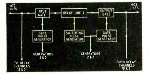
Fig. 2. Simplified block diagram of one of the delay channels. The input gating generators are controlled by the 675-line sync pulses and the output gates from a 5 : 3 count-down circuit operated by these pulses.
