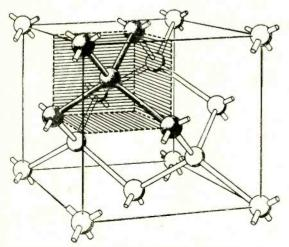
Fig. 1. Atomic structure of a germanium crystal.
