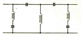
T.C.C. printed "i.f. breakthrough" filter.
