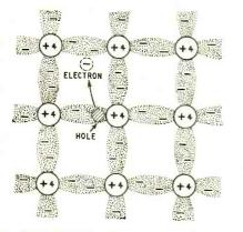
Fig. 3. "Hole" left by electron having "jumped" out of its place, due to thermal or photo effects.
