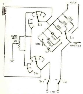
Fig. 2. The addition of two wafers to switch S3 in Fig. 1 permits the use of a single calibration for the ratio-arm scale.
