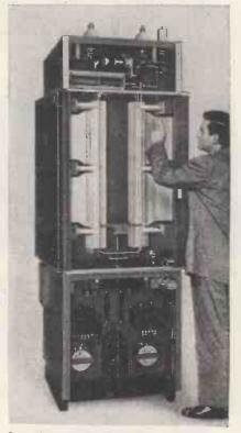
Rear view, power output section showing PA tuning and output coupling unit.
