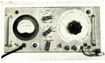
Layout of controls on the front panel. Black and red leads are used to indicate the polarity of the test clips.
