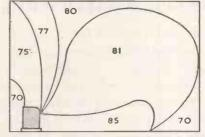
Fig. 2 Heat zones produced by a forced convection heater, the "H.M.V." 2 kW Cavendish Heater. Note the even temperature gradient throughout the entire room, with the warmer air zone at floor level. These figures were plotted from actual tests taken in a room measuring  $14' \times 11'3' \times 8'$  high (1,265 cu. ft.), with a semi-circular bay containing 5 windows.
