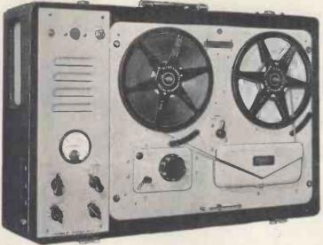
The amplifier, speaker and case, with detachable lid, measures  $8\frac{1}{2}$  in. x  $22\frac{1}{2}$  in. x  $15\frac{3}{2}$  in. and weighs 30 lb.
