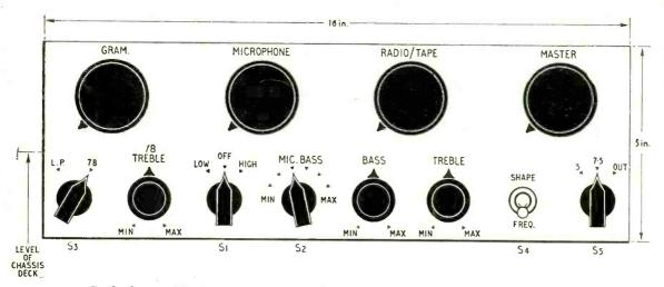
Fig. 9. Suggested front-panel layout corresponding to the under-chassis construction shown in Fig. 8.
