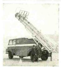
A PARABOLOID four feet in diameter is mounted on top of this 60-ft mobile extensible mast which the B.B.C. has recently introduced for television outside broadcasts. The aerial, which can be remotely rotated through 360°, can be adjusted to within + I°. When extended the mast is self supporting but provision is made for stay wires if needed.
