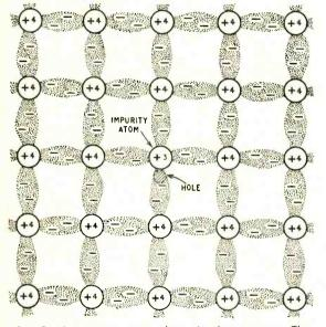
Fig. 5. An acceptor atom shown in the structure. The "hole" diffuses away from the parent atom leaving it with four orbital electrons. In these circumstances, which are normal, the acceptor atoms have a resultant negative charge.
