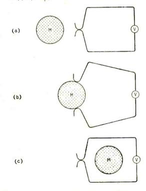
Fig. 3. M is a metal bar magnet which is pushed through the jaws of a spring clip forming a closed circuit. V is a sensitive voltmeter or galvanometer. Does it give any sign while the magnet is being inserted into the circuit? If not, why not? See Fig. 4.
