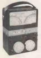
D.C. Milliameter measuring only 5in across, yet retaining a scale length of 9in.
