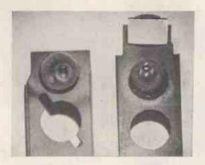
This illustration shows the pronounced pip and crater formed on the contacts of a slow make and break switch after only 7,000 operations at 230 volts, 3 amps. A.C.
