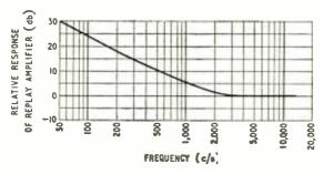
Fig. 2. Recommended ploybock characteristic for use with H.M.V. tape recordings.
