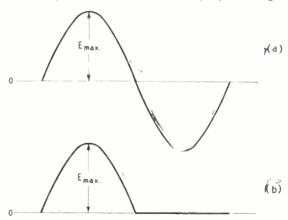
Fig. 2. The voltage waveform (a) delivered by the generator, and (b) appearing across the load resistance,  $R_{\rm L}$ . (b) is just the first half-cycle of (a), followed by no voltage for the next half-cycle.
