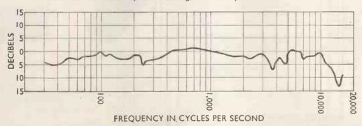
Overall frequency response of the complete equipment, comprising L.P. record, specified pick-up, Osram 912 amplifier and G.E.C. Metal Cone Loudspeakers in octagonal loaded port-cabinet.
