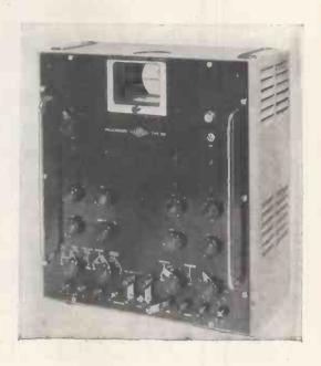
THE OSCILLOSCOPE CAMERA TYPE 758 is designed specifically for use with Airmec Oscilloscopes. It may be used for single shot photography or continuous recording, and a motor with variable speed gearing is included for the latter purpose. The cassettes will accommodate 100 feet of 35 mm. film or paper and a footage indicator shows the amount of film used.
