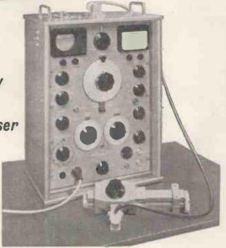
frequency modulated, and its level can be varied from +6 to -115 dB relative to 1 mW. The measurement range of the *power meter* is from +47 to -10 dB relative to 1 mW. The sensitivity of the *spectrum analyser* section is sufficient to allow its use with transmitter mean powers as low as 1 watt. The *waveguide coupling components* supplied with the Test Set include a switched two-way directional coupler for measuring v.s.w.r.
