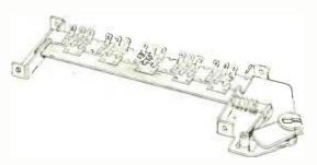
Slide switch designed by Plessey for use in a.m. f.m. receivers.
