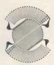
Technograph patents throughout the world now cover various alternative processes including the basic technique of making electrically conductive patterns by either the etching of metal foil previously laminated to any of the various types of insulating base, or the etching of foil patterns from metal insulated on one side by means other than laminating and bonding. These patents, together with numerous applications still pending, cover many fundamental aspects of the new technology.
