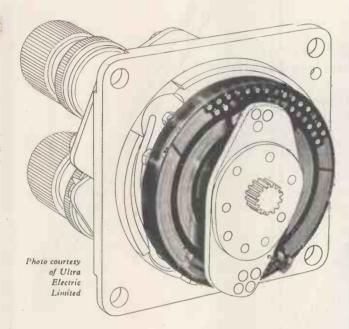
This selector unit (part of the Ultra Jet Pipe Temperature Control System) controls the temperature of the exhaust gases of a turbo-jet aero-engine.
