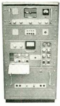
Pye PTC931,941 4-channel h.f. ground transmitter-receiver.
