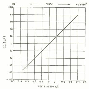
Fig. 4. Output characteristic of magnetic modulator.
