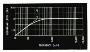
Fig. 1. Recording characteristic representative of pre-war practice. Bass amplitude is restricted to permit of reasonable groove spacing.
