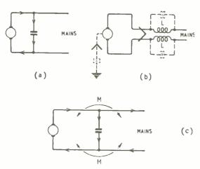
Fig. 3. (a) A capacitor shunted across the motor terminals confines most of the interference to the motor circuit. (b) A poir of inductors limits the magnitude of asymmetric interfering currents. (c) Interfering currents may by-pass the capacitor due to mutual inductance between connecting wires.
