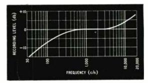
Fig. 2. A moderate degree of top lift in the recording characteristic gives an improvement in the reproduced signal-to-noise ratio.
