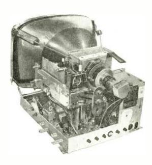
Ultra chassis. The tuner is mounted on the near side so that the controls project through the side of the cabinet.
