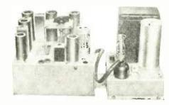
Dynatron FMI tuner and power supply unit.
