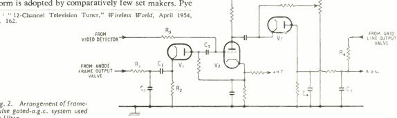
Fig. 2. Arrangement of framepulse gated-a.g.c. system used by Ultra.
