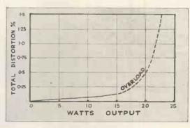
Linearity and overload of the QUAD II amplifier
