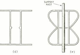
of a slot aerial is not a new idea and is, incidentally, the subject of a B.B.C. patent application (No. 19736/51). I should imagine that the single reflector illustrated by Mr. Dent achieves gain in the horizontal plane at the expense of the vertical polar diagram and that it would be better to use two rods, stacked half a wavelength apart and approximately level with the ends of the slot.
