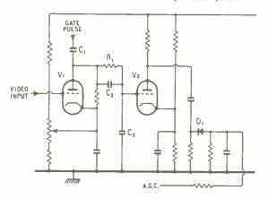
Fig. 3. Murphy line-pulse gated-a.g.c. circuit.
