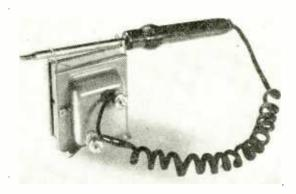
The iron on a rest fixed to the transformer
