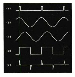
Fig. 4. Waveforms in the circuit of Fig. 3. The input sync pulses are shown at (a) and the output of the filter at (b). The phase-shifter and the squarer produce the changes indicated at (c) and (d) and the final differentiation produces the new sync pulses (e).
