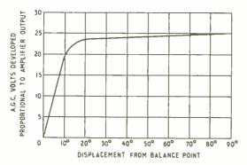
Fig. 5. Automatic gain control characteristic.
