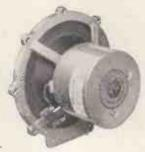
IDLE · BRADFORD · YORKS TELEPHONE : IDLE 1235/6 A highly efficient treble unit for use at frequencies above 3,000 c/cs. Flux density 13,000 lines. 1in. centre pole. Aluminium voice coil. 3, 6 or 10 ohms. Baffle opening 3½in. diameter. Price 100/-. Plus 33/3 Tax.
