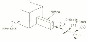
Fig. 10. Elementary crystal transducer illustrating the modes of applying stress open to the pickup designer: (1) compression, (2) cantilever, (3) torsion.
