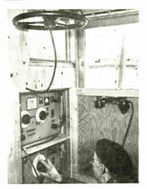
Renown-Guillemot-Seapilot radio-telephone and directionfinding equipment introduced by Marconi Marine.
