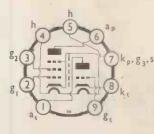
LZ3 19 Triode pentode designed for use as a frequency changer following the B319 cascode amplifier. The LZ319 operates efficiently at H.T. voltage of 170-180, and gives a high conversion gain with standard circuitry.
