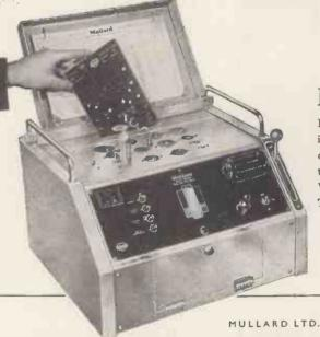
Industries which deal extensively with radio and other electronic equipment are finding the Mullard High Speed Electronic Valve Tester ideal for routine checks. instrument provides the quickest method of checking large quantities of valves, and can be operated if necessary by nontechnical personnel after only a few minutes' instruction.
