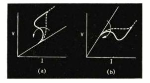
back is varied. To do this, though, you must drive the single-valued co-ordinate with a "stiff" source, which means that to plot Fig. 4(a) we apply a sweep voltage and pick off the current produced, while to plot Fig. 4(b) we apply a sweep current and pick off the voltage. If you sweep the emitter voltage in Fig. 2 the current will simply cut the corners and will never show you the negative resistance region at all.
