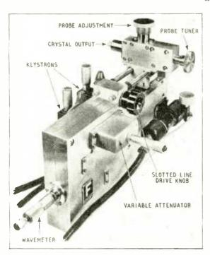
The method of manufacture greatly reduces costs (it is said to take one-third of the time required to produce a conventional test bench); it makes possible a more consistent product; it facilitates internal inspection and accessibility; and because there is no
