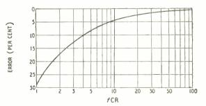
Fig. 9. Approximate low-frequency error curve calculated by Bell's method for series-diode circuit on the assumption that  $R_{\rm s}$  +  $r_a$  is negligible.
