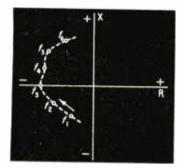
Fig. 7. The locus of the complex impedance R+jX as the frequency is increased from  $f_1$  to  $f_8$ . This particular example shows a negative resistance.
