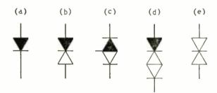
Fig. 2. A convention for junction transistors. (a) rectifier, (b) p-n-p transistor, (c) n-p-n transistor, (d) p-n-p-n compound transistor, (e) p-n-p symmetrical transistor.
