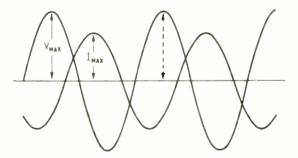
Fig. 2. In the Fig. I type of diagram, relative magnitudes are compared by noting the dimensions marked—the peak values—and phase by the distance between (in this example)  $I_{max}$  and  $V_{max}$ , compared with one whole cycle.
