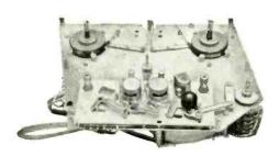
M.S.S. Model X tape mechanism.
