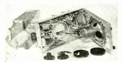
An unorthodox form of construction is employed, for, as can be seen, the loudspeaker is mounted on a hinged cover enclosing the underside of the receiver chassis with the magnet protruding through the receiver section. This
