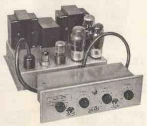
This 10-watt amplifier maintains, in every respect, the world-renowned LEAK reputation for precision engineering, fine appearance, and fastidious wiring. The Pre-amplifier will operate from any well known pick-up, whether crystal, moving iron or moving coil. Provision is made for Tape Recorder and Playback and as an exclusive feature, readily accessible jacks are provided on the front panel for instantaneous use.
