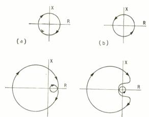
Fig. 8. Typical plots of R and X for, (a) and (c), series type and, (b) and (d) shunt type negative impedances.
