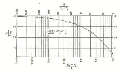
Fig. 5. (Left) Graph showing the efficiency of rectification V,  $E_{max}$  as a function of series resistance in the series-diode rectifier. It also applies exactly to the shunt-diode circuit if either  $R_s$  or  $r_a$  is zero, and nearly exactly for any values of  $R_s$  and  $r_a$  within the limits of the curve shown. The prints relate to experimental readings with the shunt and series circuits.
