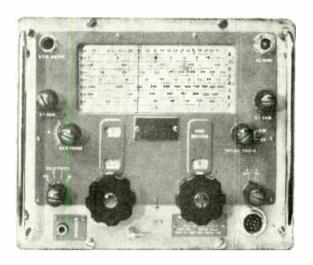
The double superheterodyne principle offers certain advantages on all but the longest wavelengths, but especially so on those below 100 metres (3 M2/s). The wider separation between the signal and the first mixer oscillator frequencies assists circuit alignment by minimizing "pulling" and, perhaps most important of all, it gives greater freedom from second-channel interference. As the table shows, the two i.f.s used in this set are 1.4 Mc/s and 460 kc/s respectively.
