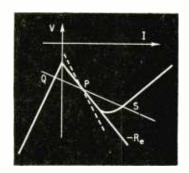
The dotted load line, for  $R'_L \le R_b$ , has only a single stable intersection, at P. Quite clearly the S-type characteristic is short-circuit stable and open-circuit unstable.
