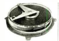
Special sine-cosine potentiometer made by Salford Electrical Instruments.
