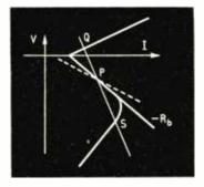
Fig. 3. The other type of negative resistance characteristic.
