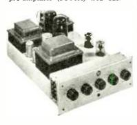
Pye Type FF91 amplifier and PF91A pre-amplifier and control unit.
