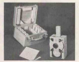
circuit in which resonance is indicated by a sensitive movingcoil micro-ammeter with crystal rectifier. It has an accuracy of  $\pm 3\%$ . For carrying purposes, a polished hardwood case accommodates the instrument and its eight plug-in coils.
