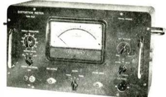
single self-contained unit. The next problem is to decide which individual harmonics are of interest, or alternatively whether the total harmonic distortion is to be measured. For our particular problems a frequency of 1,000 c's was chosen, and it was decided to provide facilities for measuring either the percentage of total distortion of that of third harmonic distortion.
