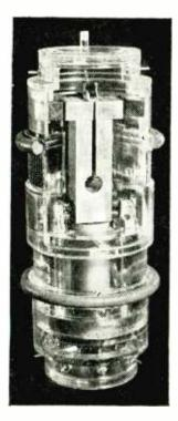
motion in the shaft of the fork. The greater the rate of turn applied to the fork the greater the amplitude of this torsional vibration. As for the direction of turn, clockwise or anticlockwise, this is indicated by the phase of the torsional vibration. With clockwise turning, an inward swing of the vibrating prongs causes the torsion blade to approach the leftpick-up hand coil. while with anti-clockwise turning an inward swing sends it
