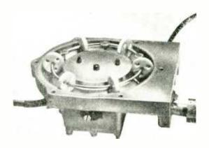
Fig. 4. The ring mixer consists of a coaxial transmission line, 1.5 wavelengths long, formed into a circle. This is an opened-up view.
