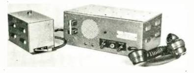
Hudson v.h.f. mobile radio-telephone installation. The unit on the left is the power supply.
