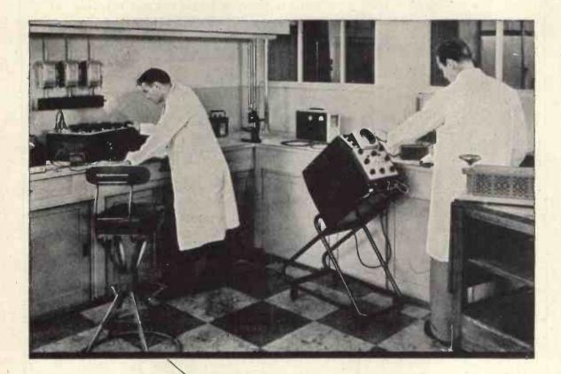
THE BENJAMIN ELECTRIC LTD. have equipped their new Research Establishment with the Cossor Double Beam Oscillograph, seen here in a section of the instrument and electrical testing laboratory where it is being used for checking wave form on control
