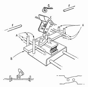
Fig. 3. Exploded view of the changeover mechanism.
