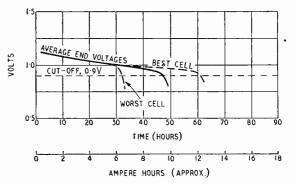
Fig. 2. Cells of another make discharged and reactivated under the same conditions. Worst cell perforated under discharge when e.m.f. was 1.05V.
