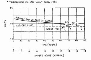
Fig. 1. Batch A. 6 cells of same make discharged 3 hours daily through 6 ohms and recharged at 0.1A for 8 hours. All cells came to an end through perforation of the cans.
