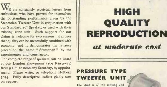
pressure type, similar to that in the 10 in. and 12 in. Concentric Duplex Units. Speech coil of aluminium wire, wound on an aluminium former, rigidly fixed to an aluminium diaphragm. Speech coil and diaphragm are at the rear of the magnet; the centre pole is hollowed out to form the commencement of the horn, in the centre of which is the 75/6 phase equaliser. Tax Free
