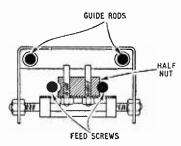
Fig. 2. Cross-section of the wire-feed carriage.
