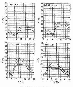
FREQUENCY BELOW WHICH COMMUNICATION SHOULD BE POSSIBLE ON ALL UNDISTURBED DAYS ---- PREDIGTED AVERAGE MAXIMUM USABLE FREQUENCY ..... FREQUENCY BELOW WHICH COMMUNICATION SHOULD BE POSSIBLE FOR 25% OF THE TOTAL TIME
