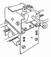
Left : Fig. 5. Details of the stops (two required) actuating the toggle changeover mechanism at the end of each layer of wire.
