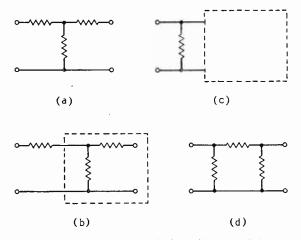
Fig. 2. In developing one dual of a ladder network (a) we take the first arm and the "rest of the network" (b), dualize the first arm (c), and then proceed to operate in the same way on each succeeding element (d).
