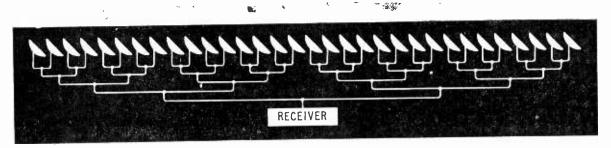
Branching system of lines connecting the paraboloids to the receiver is arranged so that the length of line from each element to the receiver is the same. Changes in line length due to temperature variations affect all elements equally and so do not disturb the phase relationships.
