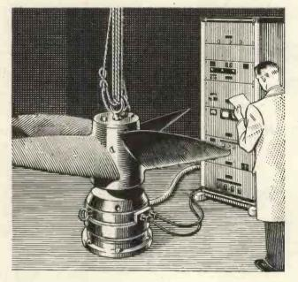
Electronic means are available by which the vibration characteristics of a propeller—be it for a ship or for an aircraft —can be analysed accurately, enabling the designer to ensure a safe component without excessive weight or unforeseen resonances. The technique has been established in the course of experience over many years.
