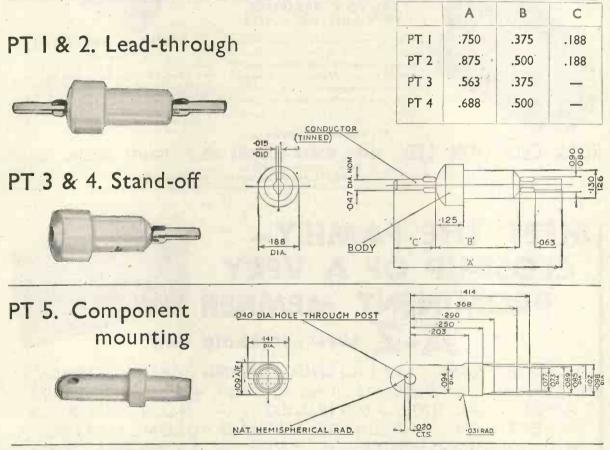
Fixing: Polytags are primarily designed for fixing with a 5 B.A. nut - PT 1-4 or an 8 B.A. nut PT 5. They are self-tapping.
