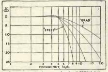
Frequency amplitude curves for the "TREBLE-3" position (5kc/s turnover). Curves of the same slopes are obtained on the other two positions turning over at Tkc/s and 9kc/s ("-2" and "-1" positions).
