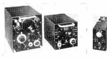
pulse-power of about 4 watts. Speech is transmitted by frequency modulation of the 6-kc/s pulse repetition frequency.
