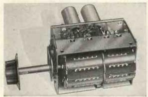
Underside view of Cyldon TV.12 "Teletuner," with casing removed.
