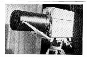
This new telephoto lens for television cameras being used by the B.B.C. has the exceptionally long focal length of 80in. Instead of the usual refracting system it uses a reflecting system consisting of a concave main mirror and a convex secondary mirror. The lens was designed by Marconi's in co-operation with Cox, Hargreaves and Thomson.
