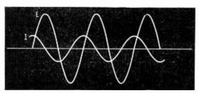
Fig. 5. Oscillograms of current through and voltage across a loss-free capacitor. Although power is flowing all the time, its direction changes twice per cycle, so the average is nil, which means that the a.c. resistance is nil.
