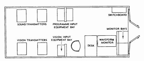
Layout of the equipment in the transmitter trailer in use at Truleigh Hill, near Brighton. Three-stack batwing transmitting aerial, supplied by Marconi's, which surmounts the 250-ft lattice mast at Pontop Pike.
