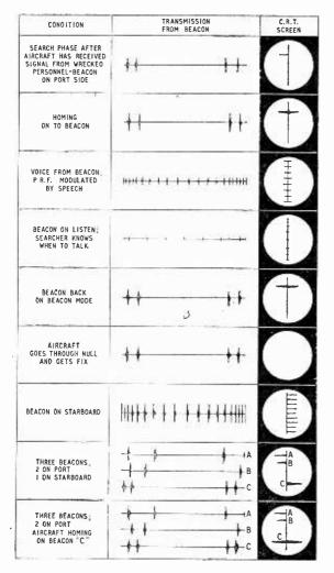
Sequence and interpretation of displayed signals on cathode ray tube in the searching craft's receiver.
