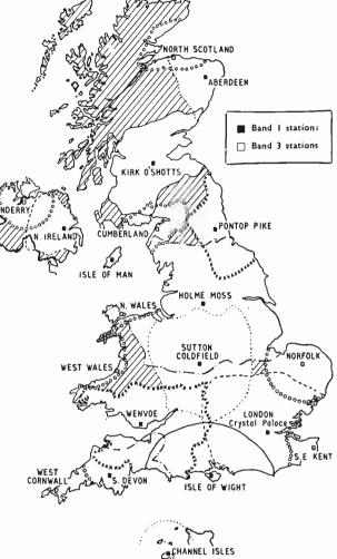
Estimated coverage of the stations planned by the B.B.C. for a single-programme service using the whole of Band I and two channels (205.5 and 215.5 Mc/s) in Band 3. Shaded areas will receive a median field strength of less than 225  $\mu$ V/m from Band I stations and less than 500  $\mu$ V/m from Band 3 stations. It will be noted that the estimated service area of the London station is based on the new high-power transmitter being erected at the Crystal Palace.
