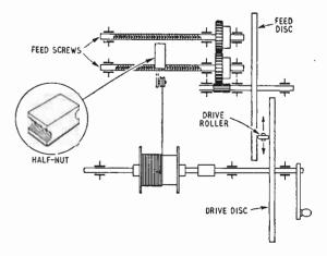
Fig. 1. Basic design of the coil winder.
