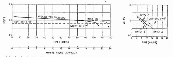
Left: Fig. 3. Batch C. Even the worst performer in this group produced current corresponding to a much greater weight of zinc than was originally contained in the entire can. Right: Fig. 4. Cells discharged under the conditions of Figs. 1, 2 and 3, but not reactivated. Voltages at the end of each 3-hours run are shown.
