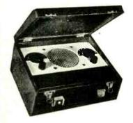
A Midget i-valve Superhet Portable Set covering medium and long wavebands.
