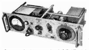
Quartz crystal activity test set shown by Salford Electrical Instruments.
