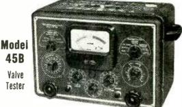
A comprehensive mutual conductance valve tester capable of measuring over 3,500 types of American and European radio valves. Supplied with a valve chart giving testing data. For use on A.C. Mains. Simple in operation. For operation from 105-125 volts and 200-250 volts A.C. supply at 40-100 List Price £25.10.0 c.p.s.
