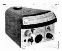
ciple and embodies a suspensiontype mirror galvanometer movement, which is critically damped magnetically.
