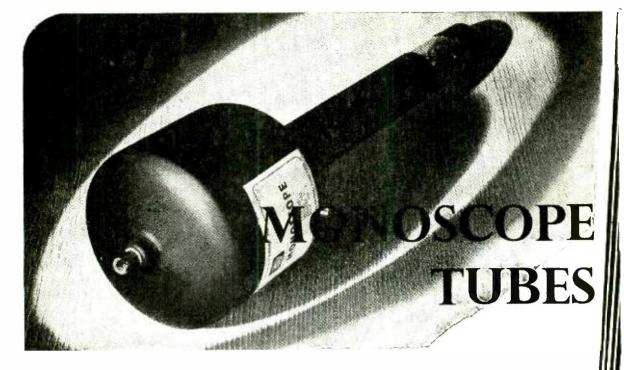
THE Monoscope is basically a simple caption scanner apparatus capable of providing a video signal derived from a fixed pattern within the tube.
