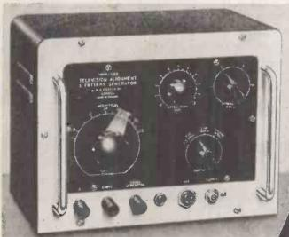
THE FIRST ENTIRELY ELECTRONIC INSTRUMENT FOR TELEVISION ALIGNMENT AND LINEARITY CHECKS
