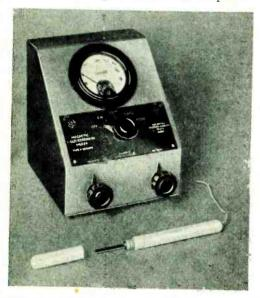
B.T.H. gauss meter, Type G, and (below) close-up of the probe, which is protected by a non-magnetic
