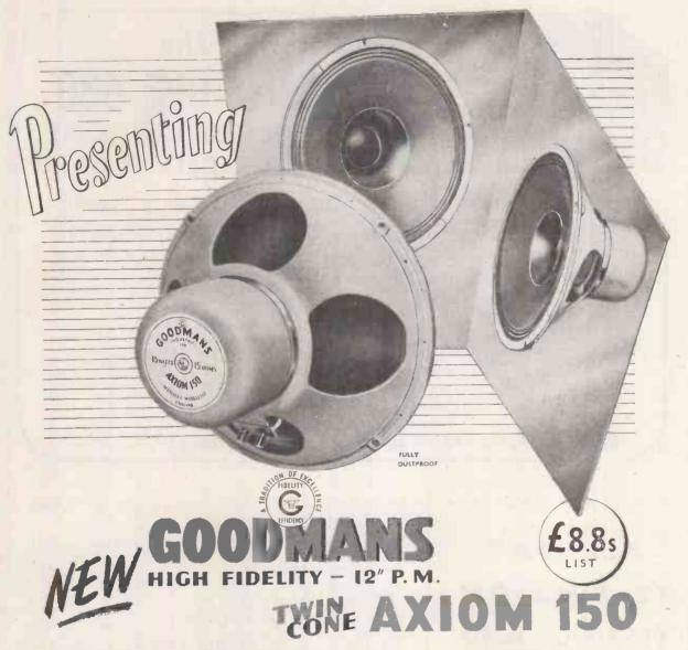
This 12in. high fidelity unit has a twin-curvilinear diaphragm (Patent No. 451754). A carefully designed magnet assembly using anisotropic material provides a total flux of 158,000 maxwells on a 13in. pole. The back cen-
