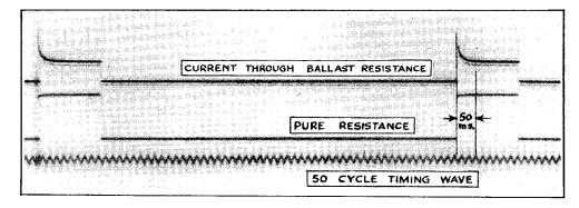
Fig. 4 .--- Behaviour of ballast resistor on make and break.
