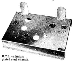
with all holes cleanly punched and fitted with valve holders and brackets for the volume and selectivity controls. Holes for the passage of wires are bushed, and the chassis is extremely rigid. It can be confidently recommended for this receiver and is priced at 10s.
