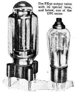
The UFC valve is a heptode frequencychanger of the Universal type. It is especially interesting in that its heater rating of 6.5 volts at 0.3 ampere enables it to be used in car radio sets where only a 6-volt accumulator is available. It is fitted with a 7-pin base and priced at 15s.
