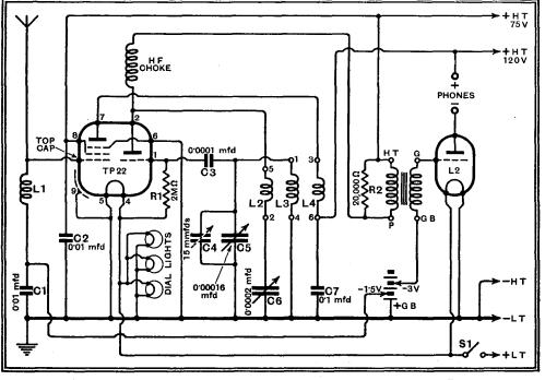
Fig. 1.—Theoretical circuit diagram of the two-valve short-wave receiver. The first valve combines the functions of HF and detector.
