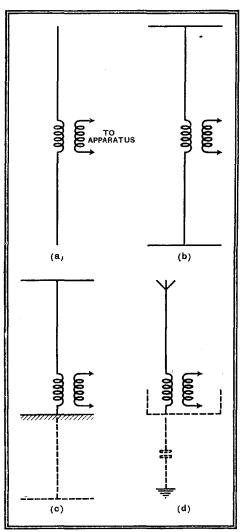
Diagrams a and b represent fundamental types of unearthed aerials (dipoles). Diagram c shows how the equivalent of b is obtained by making the earth act as one-half of the a set a set through stray capacity without any visible connection.
