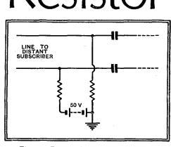
Fig. 3.—Bridge circuit used in central battery exchanges.
