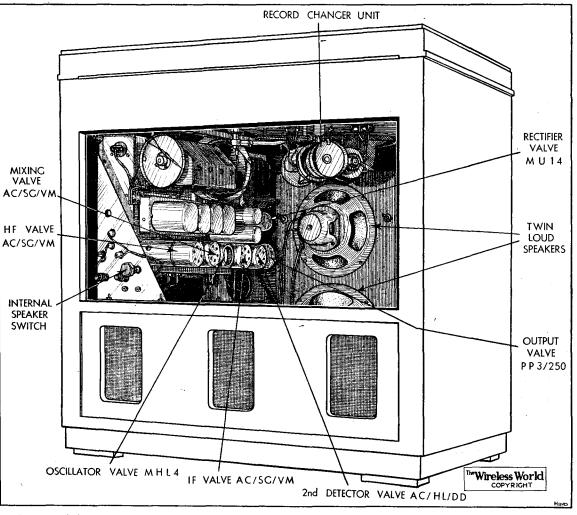
The chassis is mounted at the side of the cabinet with the controls passing vertically through the motor-board. Twin loud speakers of different diameters are used to cover the frequency range.
