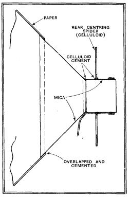
Cross-section of diaphragm showing details of construction.
