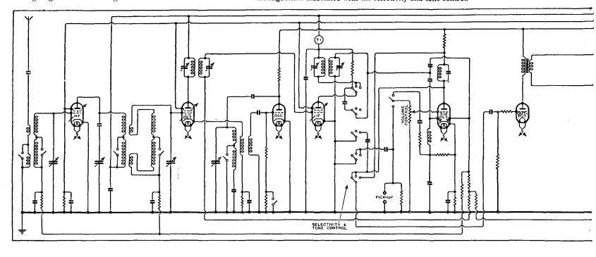
LTHOUGH moderate in price by comparison with some of the more ambitious products of this firm, the Model 704 nevertheless incorporates most of the features upon which the R.G.D. reputation has been built. A radio receiver chassis of advanced design gives wide range with variable normal output transformer connections, which increases selectivity at the expense of slight side-band cutting; but the LF circuits remain the same as in position r.
