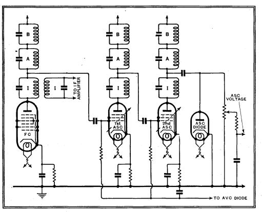
Fig. 3.—The ASC amplifier, showing how it is coupled to the frequency-changer. The ASC voltage controls the selectivity-modifying circuits, which are not shown here.
