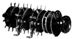
Bulgin five-way multi switch showing two units with brackets and one without, assembled on a 6-in. shaft.
