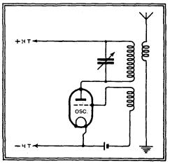
Fig. 1.-Basic valve transmitting circuit.
