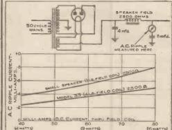
One method of comparing the relative efficiency of two field coils is to measure the amount of A.C. ripple which is present in the output, after the field coil has been used as a choke in a normal circuit. A comparison is made in the diagram between the MAGNAVOX MODEL "33" with its large field structure, and a standard type of speaker with about one pound of copper wire in the field coil, and correspondingly less iron.
