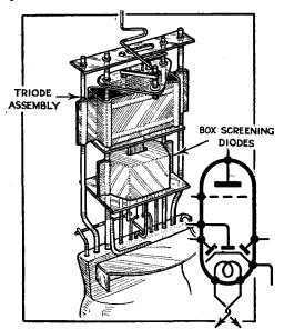
Electrode assembly of a multiple valve (triple-diode-triode).
