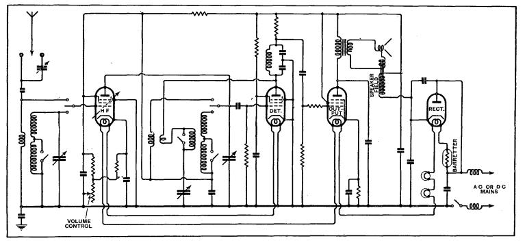
Complete circuit diagram. The aerial coupling is aperiodic on short waves, and separate reaction windings are used for the normal broadcast wavebands and the short-wave range.
