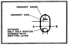
Fig. 5. The "non-radiating" valve has two false grids A and B, and a cathode which is only half coated.
