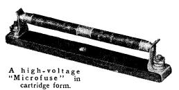
These extraordinarily delicate fuses are made on the same principle as "Microfuses" of more normal ratings, and the fusible element consists of a gold film, but in the present case this film is only about five millionths of an inch thick.
