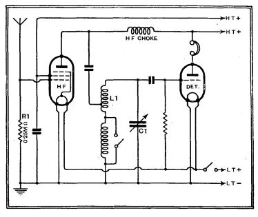
Fig. 1.-The original circuit; reaction is omitted for the sake of simplicity.
