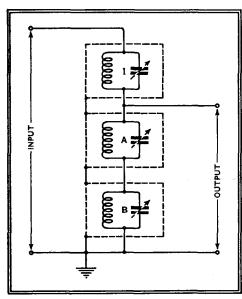
Fig. 2.—Rejector circuit filter employed in the ASC amplifier.
