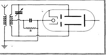
with a push-pull input circuit, and if the two deflector plates be joined together a conventional input circuit can be used. HF currents then appear in the anode circuit, and it is quite possible to obtain reaction effects. The curves of Fig. 4 show at A the input/ output characteristics, and at B those of an HF pentode,
