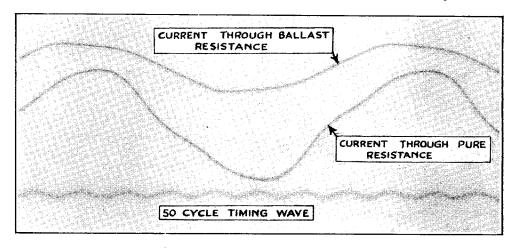
Fig. 5.-Illustrating action of ballast resistor on 7-cycle wave.
