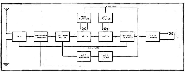
Fig. 7.-Superhet embodying two stages of anti-regenerative ASC. In all, four extra variable-mu valves and a diode are necessary.
