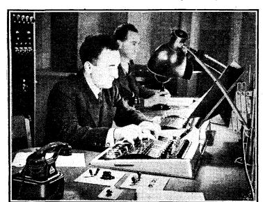
MODERNISING THE D.C. PANEL. Two new dramatic control panels which have just been installed in Berlin Broadcasting House. The sliding controls greatly facilitate the handling of multiple studio outputs by one man. Economy of space is another great advantage.
