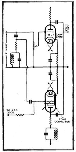
Fig. 8.—A stage of "ATC," a form of ASC accomplished wholly in the LF amplifier.
