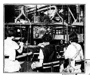
(Above) The exhausting plant. On the left the "getter" is being fired with an HF heater coil. (Right) Electrically
