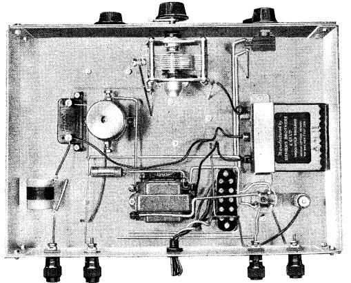
The under side of the chassis, which measures 3in. deep, accommodates the reaction condenser, HF choke, sundry other small components, and the bulk of the wiring, also the small aerial coil.
