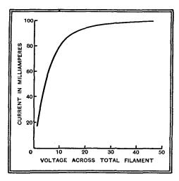
Fig. 2.—Characteristic of 100 mA. Siemens ballast resistor.
