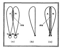
Fig. 1.—Polar diagrams illustrating the overlapping of fields of radiation from adjacent beacon stations.
