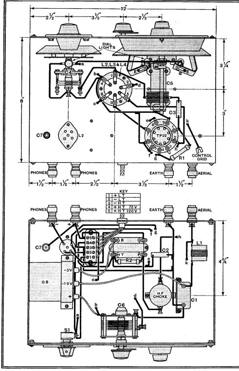
Practical wire plan and lay-out of the components on the baseboard. A metal chassis and panel is used, the size of the latter being 12in.  $\times$  10in.
