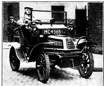
RADIO ON "OLD CROCK." Mr. E. A. Marshall, of Edgware, with his 1904 De Dion Bouton which he equipped with a Marconi car radio set for the Old Crocks' run to Brighton on Sunday last. The aerial was placed beneath the running board.
