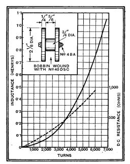
Fig. 2.—Coils of inductance greater than 0.4 are wound on a former §in. wide henry and the full-line curve provides the winding data. The DC resistance is given by the dotted-line curve.
