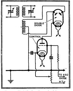
Fig. 5.—Variable-damping selectivity control, using a triode and full-wave rectifier.
