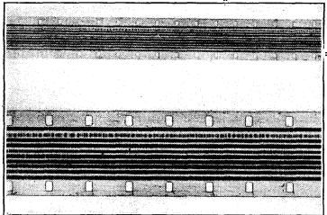
from 30 to 10,000 cycles per second can be reproduced when the strip travels at a speed of about 90 ft. per minute. By employing a rapid development and fixing process, the sounds can be played back within 15 to 25 minutes with very little loss of quality and, of course, no needle scratch.
