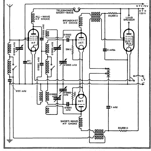
Fig. 4.-The final circuit, with values of principal components.
