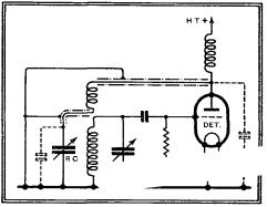
Fig. 2.- The screening of reaction leads will cure instability due to stray couplings, but will add to the minimum capacity of the reaction condenser.
