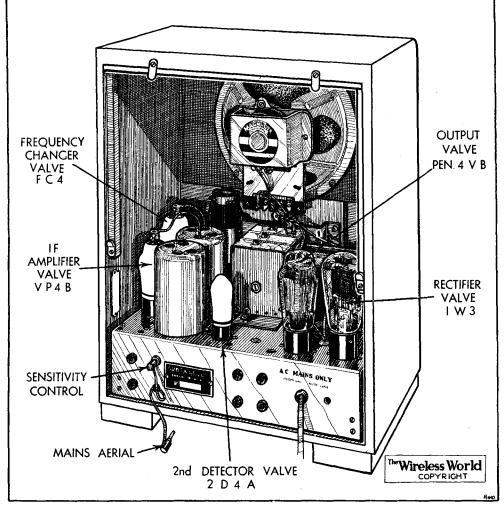
General view of the interior of the set. Two flexible leads are provided at the back of the chassis, one for a mains aerial connection and the other to give a fixed reduction of sensitivity.
