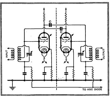
Fig. 4.—Valve-coupled band-pass filter. The coupling condensers CC are of very low capacity, and screening is very thorough.
