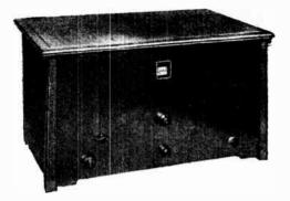
FEATURES. Four-valve circuit with one H.F. slage transformer coupled to regenerative grid detector, which in turn is linked by a driver stage to a Class "B" output valve. Undistorted oulput, 2 watts; average H.T. consumption about 10 milliamperes. Single-tuning control with illuminated dial and wavelength calibration. Price: Set of components, with valves, £12 17s. Without valves, £10 10s. 9d. Cabinet and baseboard, 30s. extra. Makers: Ferranti Ltd., Hollinwood, Lancs.
