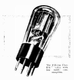
120 the total quiescent feed current of the output valve will be 2 milliamperes, the power output 1 watt, the driver transformer overall ratio 2 to 1, and the anode-to-anode load 17,000 ohms. Using the P.220 valve as a driver and assuming an H.T. voltage of 120, the total quiescent feed current of the
