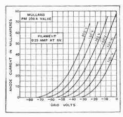
Characteristics under working conditions: A.C. resistance 1,410 ohms, amplification factor 3.1, mutual conductance 2.2 mA./voit.
