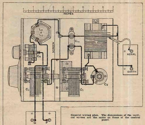
band pass unit, as full details were given in the description of the "Regional One" receiver, to which the reader is referred. It would seem fairly safe to predict that once a ganged filter has been pressed into service and the remarkable selectivity and quality experienced, single uncoupled circuits will not be employed again.
