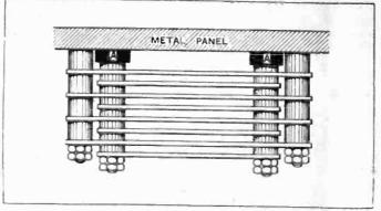
Fig. 2.—Method of supporting the plates of an air dielectric condenser and used to compare the material with ebonite.
