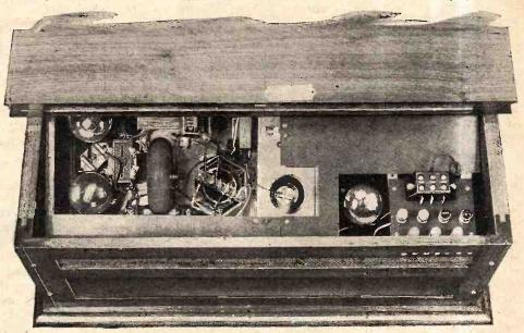
This illustration shows the mains smoothing and rectifying equipment on the right. In the left-hand compartment the H.F. components, including the toroidal transformer, can be seen.
