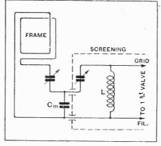
Fig. 1.—A frame aerial as part of a capacity-coupled filter.
