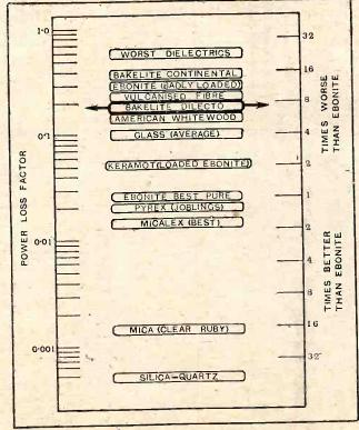
Fig. 1.—The relative power factor of Bakelite in comparison with pure chonite is shown on the above chart,
