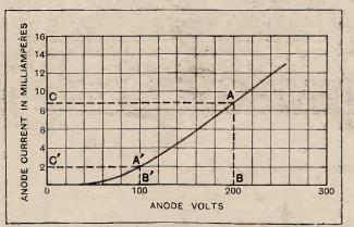
Fig. 1.—The anode voltage/anode current curve of a valve obtained with the grid potential fixed. At 200 volts the apparent or D.C. resistance is given by  $\frac{AC}{AB} = \frac{200}{0.0088} = 22,700$  ohms. At 100 volts the apparent resistance is  $\frac{A^4C^4}{A^4B^4} = 50,000$  ohms. Fig. 3 shows how the effective A.C. resistance is obtained.
