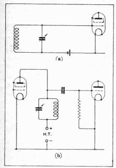
Fig. 2.—Where to look for losses in tuned circuits.
