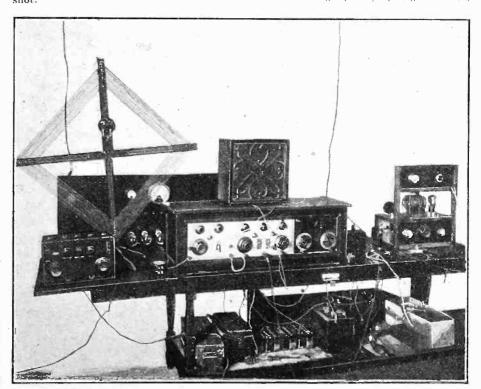
CT 2AG owned and operated by Fernando Hinte at Gorreana, San Miguel, Azores. The transmitter, on the right, is a Mesney using about 20 watts to a Philips JB004/10 valve and coupled to a full-wave 42-metre Hertz aerial. The receiver in the foreground is an 8-valve superheterodyne.
