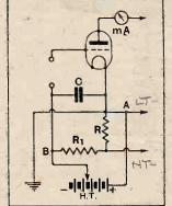
nect A to the positive of a high-tension battery and vary the position of the lead to B so that no change in the anode current occurs. When this point is found the voltage applied by the battery is, of course, equal to the free bias. Measurements may even be made without a milliam-meter by substituting a loud speaker, but are somewhat less easy.
