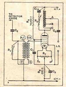
Fig. 1.—The "Power Pentode Two" with an indirectly heated pentode in place of the original directly heated output valve.
