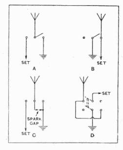
Fig. 1.—Methods of connecting aerial safety switches.
