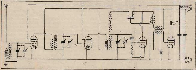
Simplified circuit diagram showing essential features of the new receiver. Trimming condensers are drawn in dotted lines.
