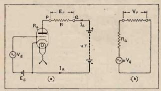
Fig. 2.—(a) A three-electrode valve with a resistance R in the anode circuit. The voltage E, developed across R is proportional to the anode current. (b) Equivalent circuit relating to the A.C. components in the anode circuit when the grid voltage has an alternating component.  $V_r$  is the A.C. component of voltage developed across R. Voltage amplification  $n = \frac{V_r}{V_g} = \frac{\mu R}{R + R_s}$ .
