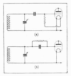
Fig. 3.—Alternative grid leak connections.
