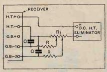
Fig. 1.—Adding a "grid bias battery eliminator" to a receiver deriving its anode current from D.C. mains.
