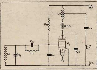
Fig. 1.—Simplified circuit diagram of one-valve loud speaker receiver. Details of the complete aerial tuning scheme and the A.C. eliminator have been omitted.
