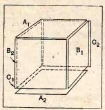
Fig. 6.—Three pairs of closed loops arranged mutually at right angles to screen a cubic space.
