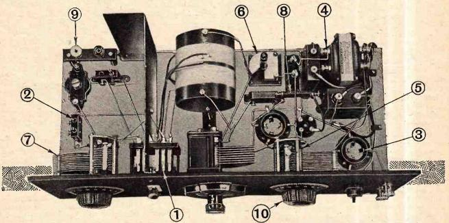
Points at which mechanical faults and electrical contact failures may possibly develop. Reference to key numbers is made in the text.
