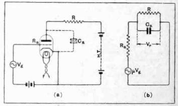
Fig. 3.—Diagrams for illustrating the effect of capacity between the anode and cathode of a valve on the degree of amplification obtained at various frequencies.
