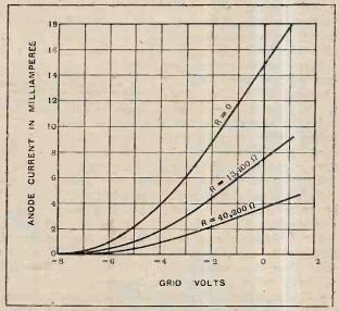
Fig. 3.—Curves showing how resistance inserted in the anode circuit affects the anode current of a valve. The A.C. resistance of the valve is 13,400 ohms and its amplification factor 36. The curves correspond to 200 volts H.T. supply throughout. The numbers attached to the curves indicate the resistance connected in the anode circuit.
