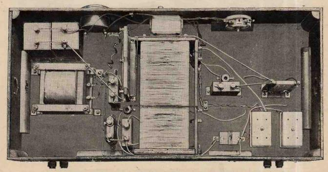
View of the underside of the sub-base showing the smoothing choke, voltage regulating resistances and the 8 mfds. condensers on the left.
