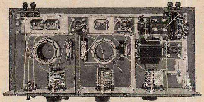
Plan view of the set with valves and screening box covers removed. The aerial-grid coil and the rejector condensers are on the left.
