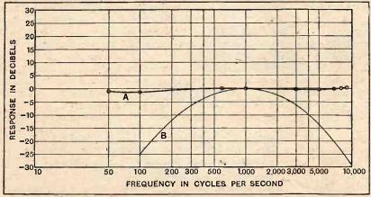
Fig. 4.—FREQUENCY RESPONSE CURVE. Special B.B.C. test transmission on 356.3 metres, June 4th, 1930. Curve A shows  $20 \log_{10} \left(\frac{v}{v_{1000}}\right)^3$  where v is the receiver output voltage and  $v_{1000}$  is the value of this voltage at 1,000 cycles per second. Transmitter modulation voltage constant. Curve B is for a small portable receiver measured under like conditions.
