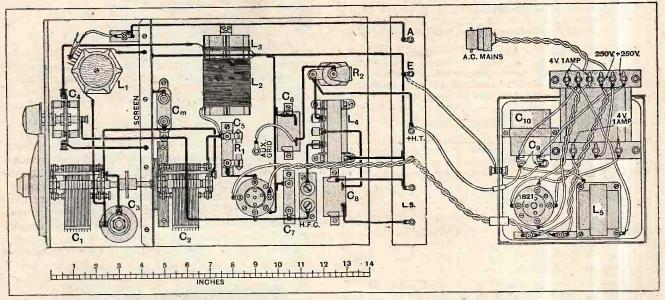
General wiring plan. The smoothing condenser C10 is held vertically above C0 by a small metal strap. The dimensions of the vertical screen are the same as those of the panel.
