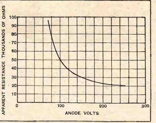
Fig. 2,—The apparent resistance of a valve obtained by dividing the anode voltage by the anode current. The curve is derived from the characteristic curve of Fig. 1.
