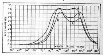
Fig. 3.—REGIONAL. M=12 turns; B, distuning 3rd circuit; C, distuning 3rd circuit and adding resistance.
