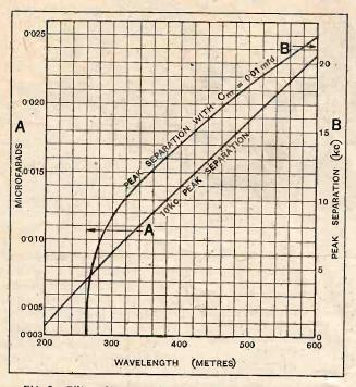
Fig. 3.—Filter characteristics of the band pass unit. Curve A to be read in conjunction with the vertical scale on the left shows the coupling capacity necessary to give the optimum peak separation of 10 kc. at any wavelength between 200 and 600 metres. Curve B to be used with the vertical scale on the right gives the peak separation at various wavelengths which will be obtained when using a fixed coupling capacity ( $C_{\rm m}$ ) of 0.01 mfd.
