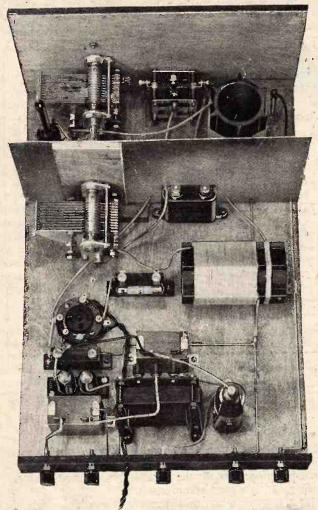
That the set is simple to construct is evident from this plan view. The centre terminal is for the H.T + connection from the climinator. The H.T. negative lead is joined to the earth terminal.
