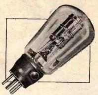
The indirectly-heated pentode—the Mazda AC/Pen. With a signal of 5 volts from a local transmission it is possible to obtain about 350 milliwatts output.
