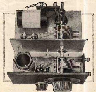
Plan view of the unit. In the compartment next to the panel are housed one member of the ganged condenser, the secondary coil with reaction winding, and the reaction condenser. A slow-motion dial will probably be found more satisfactory for controlling the ganged condenser.
