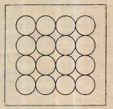
Fig. 4.—A series of loops arranged to screen a plane area from an alternating magnetic field.
