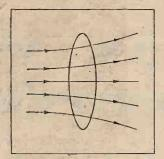
Fig. 3.—The magnetic field threading a conducting loop is opposed by the current which it induces in the loop.
