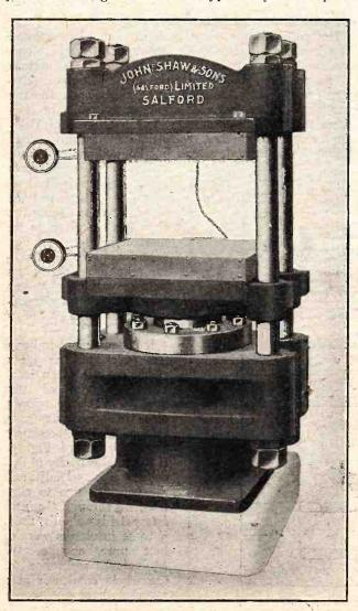
A 50-ton hydraulic moulding press, by John Shaw and Sons (Salford) Ltd., used in the manufacture of Bakelite mouldings.
