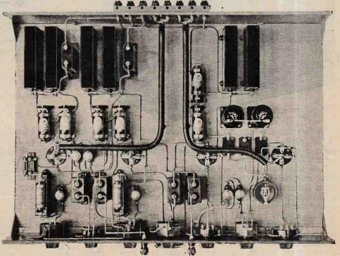
. Underside of the push-pull detector and first L.F. amplifier unit.
