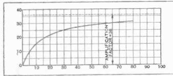
Fig. 1.—Calculated voltage amplification obtained for a valve with  $\mu=36$  and  $R_0=13,400$  ohms for various values of resistance in the anode circuit.
