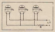
Fig. 1.—Illustrating the danger of over-running filaments when they are connected in parallel across a high-voltage source of supply.
