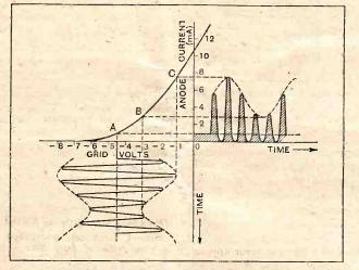
Fig. 4.—Diagram showing how the anode current varies when a modulated H.F. voltage is applied to the grid of a valve biased to operate on the lower bend of its anode characteristic curve.
