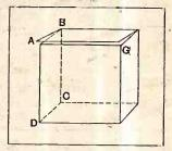
Fig. 7.—An incomplete screening box in which only the end surfaces are effective in screening fields perpendicular to A, B, C, D, until contact is made along the edge A G.
