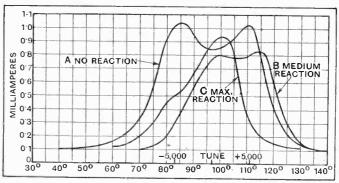
Fig. 6.-REGIONAL. M=12 turns. Showing effect of reaction.
