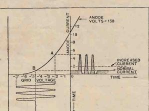
Fig. 3. Diagram showing the rectifying properties of a three-electrode valve. When working on the lower bend of an anode characteristic curve, an alternating voltage causes a change in the D.C. component of the plate current.
