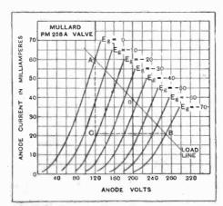
Anode volts/ahode current curves of the P.M.256A. From these the maximum undistorted power output, the optimum grid bias and the best loud speaker impedance (load line) can be found.
