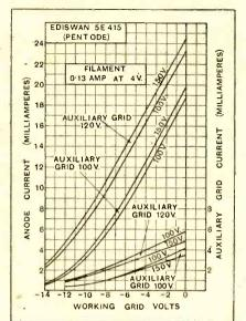
Average values, A.C. resistance, 59,000 ohms; amplification factor 83; mutual conductance, 1.4mA./volt, under normal working conditions.
