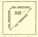
Fig. 4.—In a well-designed coil the phase angle is nearly 90° and the coil and condenser currents are nearly 180° out of phase. The slope in this diagram represents coil reactance coil resistance.
