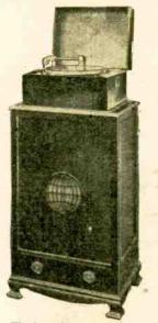
The Igranic electrically re-producing gramophone. In-directly heated cathode valves are used in the early stages.
