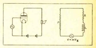
Fig. 7.—Diagram showing equivalent circuit of valve and loud speaker. V is the voltage of the fictitious alternator; ρ the internal A.C. valve resistance of loud speaker, and L the effective inductance of the loud speaker.
