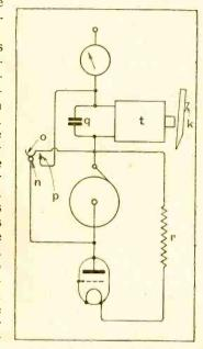
Anode circuit of the Colvergraph. The resistance provides the current for the threshold trigger adjustment. The use of a relay is abandoned. Only a single switch-over contact is needed.
