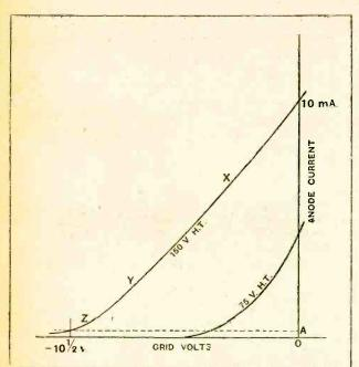
Fig. 3.—Two valve characteristics for typical modern anode bend detectors such as the PMD or DEL series. The 150-volt curve is sensibly straight for the greater part of its length whilst the 75-volt curve has no straight portion and is not suitable for anode bend detection.
