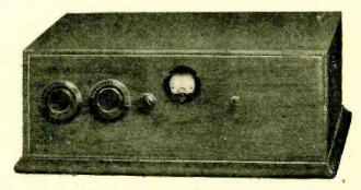
A receiver which was exhibited by Messrs. Ferranti at the last Olympia Exhibition. An anode bend meter and a post-detector volume control are incorporated.
