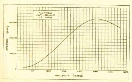
Impedance curve of the R.I.-Varley Multi-Cellular H.F. choke; external capacity 8 micro-mfd.
