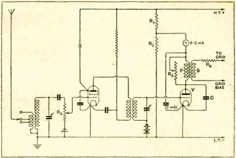
Fig. 7.—A suggested circuit to create large inputs for an anode bend detector. Constant maximum input without running into grid current is assured by the milliammeter, while the volume control R3 prevents overloading of the third valve (not shown).
