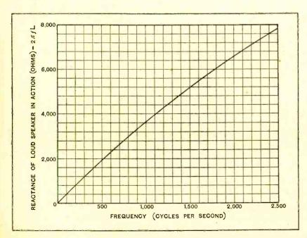
Fig. 2.—Curve showing reactance  $(2\pi f L)$  of Lion loud speaker at various frequencies.
