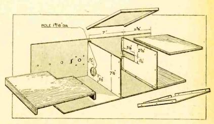
Fig. 3.-Construction of metal screens and baseboards.
