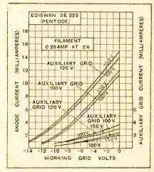
Average values, A.C. resistance, 83,000 ohms; amplification factor, 83; mutual conductance, ImA./volt; under normal working conditions.
