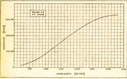
Impedance curve of Bulgin H.F. choke; external capacity 8 micro-mfd.
