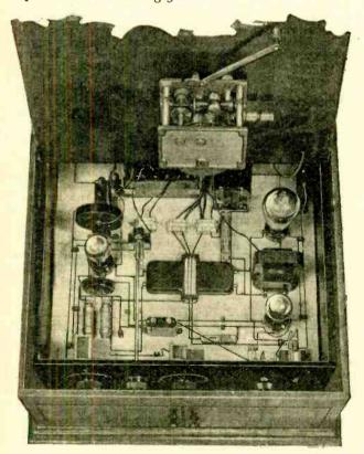
The arrangement of the receiver-amplifier components and wiring can be seen in the above photograph taken with the turntable platform raised.
