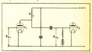
Fig. 5.—In this amplifier R fulfils exactly the role of the tuned circuit in Fig. 4; the two may be treated in exactly an identical manner.
