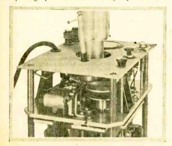
Close-up view showing the trigger release and driving pinion.
