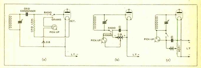
Fig. 1 .- Converting the detector for amplification: methods of connecting a pick-up in its grid circuit.
