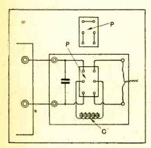
Method of switching a smoothing choke in a D.C. eliminator. (No. 300,383.)
