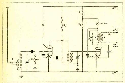
Fig. 8.—A suggested circuit containing a screen-grid valve followed by an anode bend detector. For local station reception pre- and post-detector volume controls ( $\mathbf{R}_5$  and  $\mathbf{R}_3$ ) are advised.
