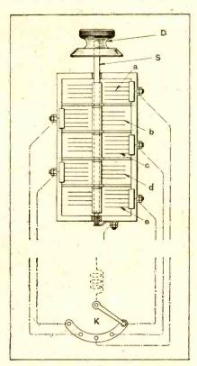
Switch-controlled selection of five differently tuned circuits. (No. 296,591.)
