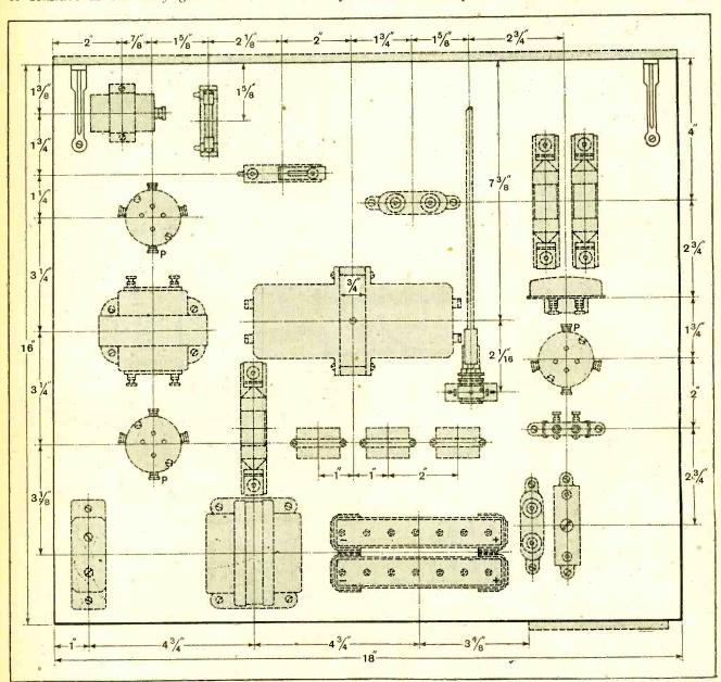
Fig. 3.-Layout of the components on the baseboard.
