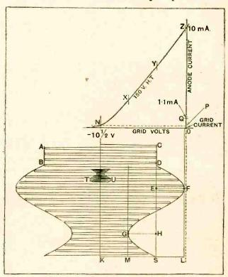
Fig. 4.—Diagram showing the application of a 10-volt (peak) 50% modulated carrier wave to an anode bend detector. Note that the total modulated swing M L is  $\frac{2}{3}$  of the peak KL.
