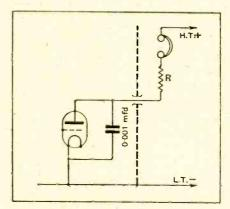
Fig. 1.—Locating instability: modified detector anode circuit.
