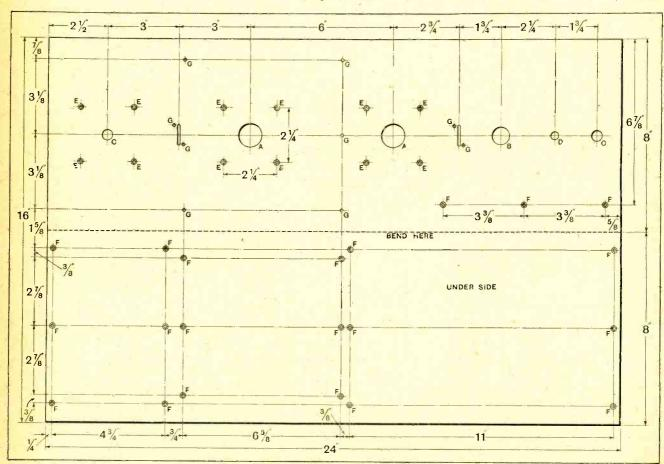
Fig. 5.—Drilling details of combined panel and base. A, lin. dia.; B, 3/4in. dia.; C, 7/16in. dia.; D, 5/16in. dia.; E, 1/8in. dia., countersunk; F, 1/8in. dia., countersunk; G, 1/8 in. dia.
