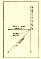
Fig. 3. — The coil current (dotted line) can be resolved into a horizontal and a vertical component.
