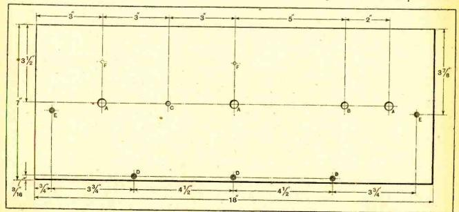
Fig. 2.—Dimensions and drilling data for the panel. A=3/8in. dia.; B=5/16in. dia.; C=3/16in. dia.; D=1/8in. dia., countersunk for No. 6 B.A. screws; and F=1/8in. dia., countersunk for No. 6 B.A. screws; and F=1/8in. dia.
