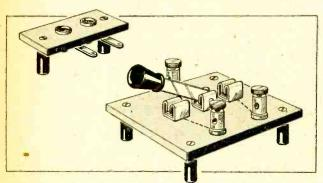
Fig. 2.-Terminal block and switch for baseboard mounting.
