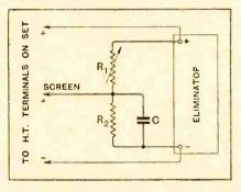
Fig. 1 .- A potentiometer for screen grid voltage control.
