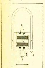
formers. Additional damping is provided by rubber inserts let into the face of each pole piece. The reproduction of frequencies up to 2,000 cycles is good, and the output shows a marked increase between 1,000 and 2,000 cycles.
