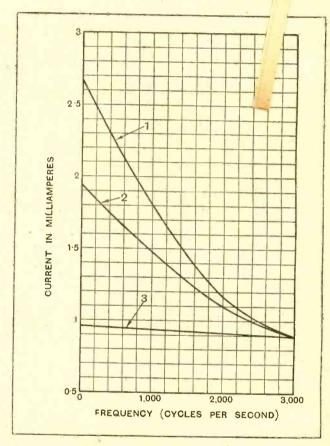
Fig. 6.—Curves showing current in the Lion loud speaker at various frequencies. Curve t = internal valve resistance = 3,000 ohms. Curve 2 = internal valve resistance = 5,000 ohms. Curve 3 = internal valve resistance = 40,000 ohms. It should be observed that there is practically no variation in current with the pentode (curve 3).
