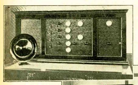
(Above) The combining receiver at the central station, and (below) the equipment at one of the substations of the receiving system.
