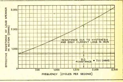
Fig. 3.—Curve showing effective resistance of the Lion loud speaker at various frequencies.
