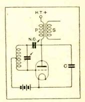
Fig. 11.—A neutralised anode bend detector. Input loading is prevented.
