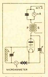
Fig. 9. — An experimental circuit to show the presence of an input load due to the interelectrode capacity of an anode bend detector.
