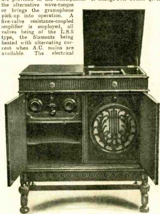
C.A.C. radio-gramophone. The gramophone motor and valves are mains operated.
