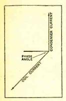
Fig. 2.— The condenser current leads the e.m.f. by 90° while the coll current lags by the phase angle.
