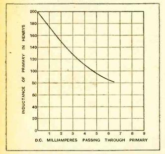
Fig. 6.—With the small anode current of 1 to 2 mA, passed by an anode bend detector the primary inductance of an intervalve transformer is not appreciably reduced. The curve is for an AF5 transformer.
