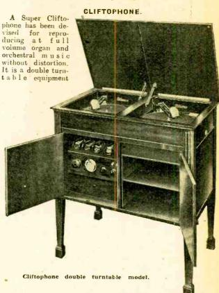
fitted with the Cliftophone pick-up, a feature of which is the provision of a parallel link motion to ensure a perfect tracking action. The equipment is entirely mains-operated, for which purpose a motor generator is supplied with appropriate smoothing circuits.
