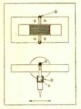
magnets, and the pick-up coil surrounds the armature. The dimensions of the unit are small, and the construction is unusually solid and compact. The output falls off gradually as the frequency is increased, and the general level requires three rather than two valves. At present the complete output of these pick-ups is being absorbed in the com-
