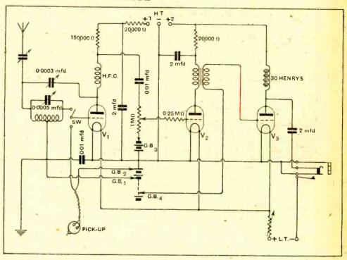
Fig. 1.—The theoretical circuit diagram. The semi-fixed aerial condenser is variable between 0.000025 mfd. and 0.0003 mfd.
