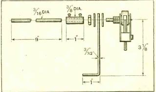
Details of the switch showing extension rod and bracket.
