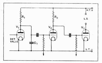
Fig. 8.—An anode bend detector followed by two stages of resistance coupling. If  $R_1$  and  $R_2$  are of the order of 2 megohms, and if  $V_1$  and  $V_2$  have high magnification factors, practically all notes at about 5,000 cycles will be lost.
