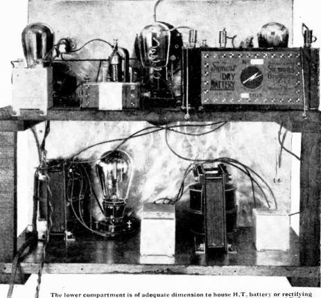
The lower compartment is of adequate dimension to house H.T. battery or rectifying and smoothing equipment for H.T. supply from A.C. mains. In the case of D.C. a potential divider takes the place of the transformer and rectifying valve.
