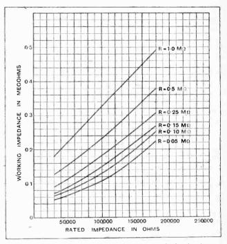
Fig. 7.—Curves showing relation between nonlinal valve impedance as given by makers and actual working impedance using various values of anode resistances.
