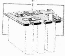
" Simpsonic " connector panel for flashlamp H.T. batteries.
