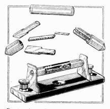
Constructional details of the Microfuse which blows at less than 100 mA.
