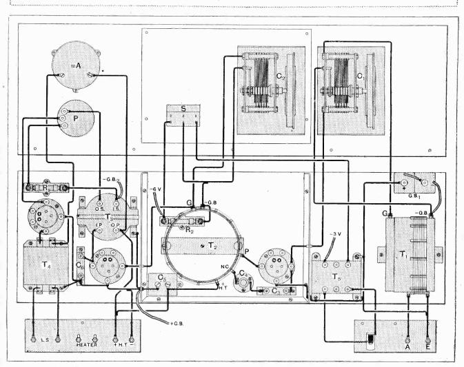
Fig. 9.-Wiring diagram. The panel and baseboard-are shown in the same plane to facilitate the tracing of wires.
