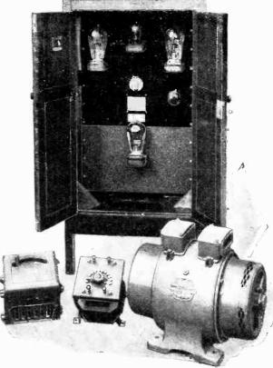
THE AMPLIFIER. The tower valve is associated with the metal fronted rectifier unit. The output of the small valve feeds the two larger valves which are push-pull connected. If the supply is D.C. a motor is used to create the necessary A.C. power input.
