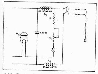
Fig. 2,—The alternative smoothing circuit to be used when the negative main is earthed. B 13
