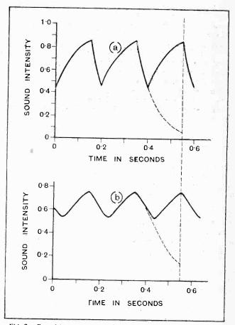
Fig. 3.—Sound intensities produced in a hall with a reverberant period of 1 second by (1) the voice (2) loud-speaker reception from a reverberant studio having a 1 second reverberant period.
