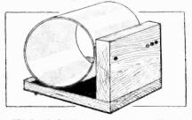
Fig. 3.—A jig for the accurate spacing of pins and sockets in the "Two-H.F. Everyman Four" type of H.F. transformer.
