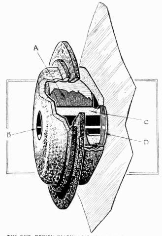
THE COLL DRIVEN DIAPHRAGM. A, field winding; B, ventilating hole through the pole; C, centre pole; D, moving coil attached to diaphragm.
