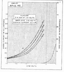
A.C. resistance = 172,000 ohms. Amplification factor = 54. Mutual conductance = 0.31 mA./volt.
