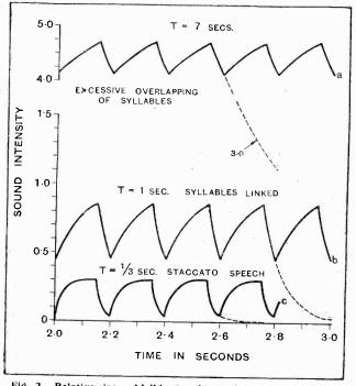
Fig. 2.—Relative rise and fall in sound intensity of single syllables issued at a rate of 5 a second under the same conditions as the curves of Fig. 1.
