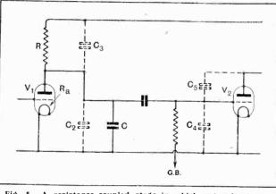
Fig. 5.—A resistance-coupled stage in which not only the incidental capacities but also the magnitude of  $R_a$  and R have a profound effect on the suppression of high notes.
