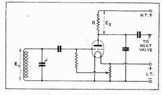
Fig. 1.—Grid rectification circuit. The D.C. volts developed across  $E_2$  were measured tor various A.C. voltages applied at  $E_1$ .
