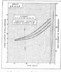
A.C. resistance = 29,500 ohms. Amplification factor = 7.7. Mutual conductance = 0.38 mA./volt.
