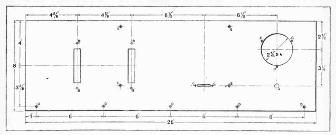
Fig. 7.—Panel dimensions. A, 3/8in. diameter; B, 5/32in.; C, 1/8in.; D, 1/8in. countersunk for No. 4 wood screws; E, 1/8in. countersunk for No. 6 B.A. screws.
