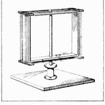
A cheap frame aerial using a wire bobbin as a bearing.
