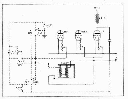
Fig. 1,--Control of a receiver from three distant points. Extension leads are shown in dotted lines. Note the earth return for loud-speaker circuit.
