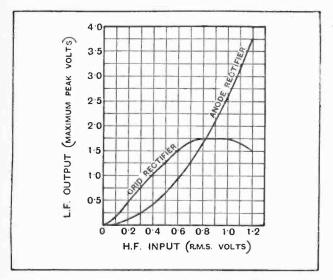
Fig. 5.—Curves showing actual L.F. peak-volts developed for various inputs of 20 per cent. modulation.
