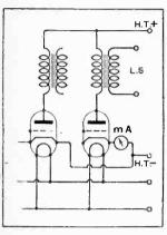
Fig. 4 .- Alternative position meter to show anode current of last valve.
