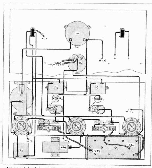
signal energy. We must perforce compromise and use a leak between 0.5 and 5 megohms, provided that the value chosen is at least ten times the value of the preceding anode resistance for these two components are virtually in parallel.
