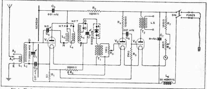
Fig. 1.—The theoretical circuit diagram. The smoothing circuit is arranged for a supply system with the positive conductor earthed.
