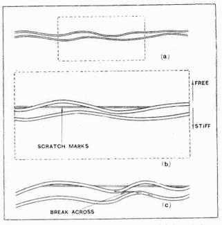
Fig. 2.—(a) Highly magnified section of record before playing.
