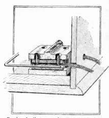
Sectional diagram showing method of fitting in receiver cabinet; holes are drilled for passing the battery leass through the back of the cabinet.
