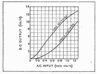
Fig. 3.—Curves showing that the superiority of D.C. voltage output from a grid rectifier diminishes as applied volts are increased.
