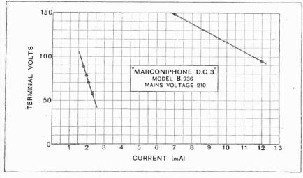
Voltage output from the Marconiphone D.C.3 under various load conditions.
