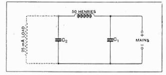
Fig. 2.—A practical smoothing clrcuit, C<sub>1</sub> and C<sub>2</sub> having the usual values. The load is that imposed by the values in the set, and by any potential divider that may be used.
