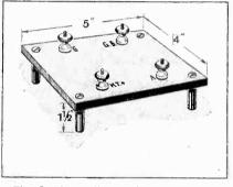
Fig. 2.—A small experimental unit for comparing the performance of various low-frequency coupling methods.
