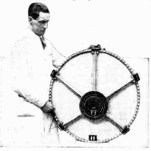
The loud-speaker consists of a stretched aluminium diaphragm of large diameter with the coil dr ve offset from the centre.
