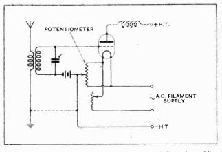
When heating ordinary valve filaments from A.C. mains additional grid bias is necessary to prevent grid current. The electrical centre of the filament is found by means of a potentiometer.
