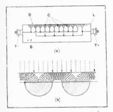
Carbon microphone with unorthodox arrangement of electrodes. (No. 278,443.)
