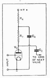
The anode feed scheme as applied to  $V_2$ . The speech currents are diverted from the H.T. battery and pass through  $C_4$  to earth.
