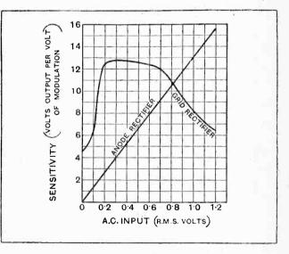
Fig. 4.-Relative sensitivities of both rectifiers measured as their response to the modulation of a carrier wave.
