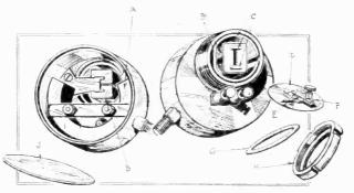
"HIS MASTER'S VOICE" GRAMOPHONE PICK-UP. A, field magnet; B, bobbins on divided end of magnet pole; C, the poles; D, the steel diaphragm; E, iron attachment for needle holder; F, brass end to prevent needles sticki g; G, oil retaining washer; H, diaphragm clamping ring; J, back cover ring.
