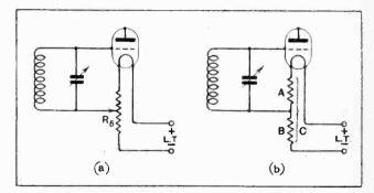
Fig. 2.—(a) Method employed in obtaining "free" grid bias from a variable resistor. (b) Use of fixed resistors in series for the same purpose.
