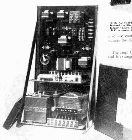
The amplifier is entirely A.C. mains operated. A screening box totally encloses the rectifier.
