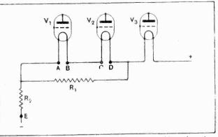
Fig. 3.-The method of obtaining negative grid bias when the filaments of the valves are connected in series.
