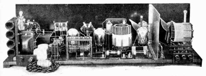
The rear view of the receiver. The current limiting resistance can be seen on the left and in the centre is the 20,000 ohms tapped resistance for supplying grid bias to the first L.F. valve.
