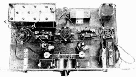
Plan view of the finished amplifier showing arrangement of parts and the easy method of wiring adopted.
