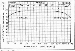
Fig. 11.—The frequency response curve of the amplifier shown in Fig. 10.
