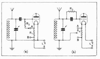
Fig. 1.—(a) Shows low potential end of grid leak connected directly to filament. (b) Shows grid bias applied through coil.
