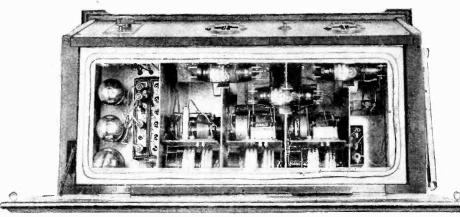
Interior of the Marconiphone Model 61. Note the braided metal beading for making contact with the metal lining of the lid.
