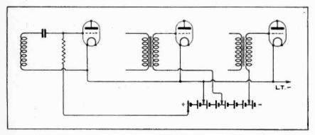
Fig. 2.-The application of positive or negative bias from a single bias battery.
