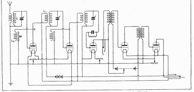
Method of balancing inter-electrode capacity by use of a plate. (No. 278,400).
