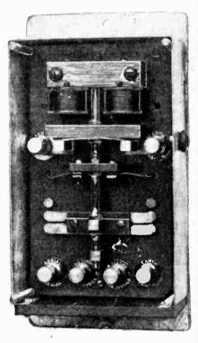
Holland automatic earthing switch with remote control.
