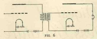
made to operate an amplifier, giving greatly magnified signals. The grid is connected through the variable inductance to the negative side of the accumulator, and is therefore neither positive nor negative
