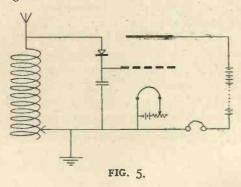
Excellent amplification may be obtained by using about 90 volts on the sheath and a 4-volt accumulator to heat the filament. Good results may be obtained by using a lower voltage on the sheath, say 30 volts, but the filament current must be reduced at the same time to ensure the valve working at the best point on its characteristic curve.
