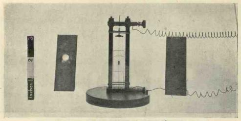
TWISTED STRIP AMMETER FROM THE INVENTOR'S LABORATORY.
