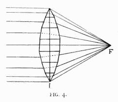
Fig. 4, the light rays being refracted towards the base of the prisms or towards the normal, as already explained; while the top half of the lens will refract all the light downwards, the bottom half will act as a series of inverted prisms and refract all the light upwards.
