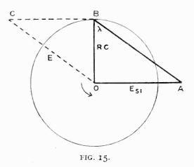
Now it will be seen that the current curve lags behind the applied E.M.F. curve, and the amount of this lag, measured in degrees, is known as the angle of lag (see Article 2, section 7).
