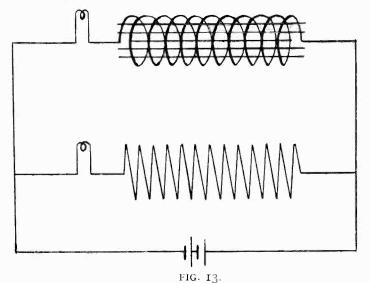
14. Growth of Current.—The E.M.F. induced in coil Q is in such a direction that the current flowing in Q will be in an opposite direction to that in coil P. This current will therefore tend to neutralize the current flowing in coil P, and consequently the current in the remaining coils will only gradually attain their maximum value. This is equivalent to the train attaining its maximum speed in our mechanical analogy.
