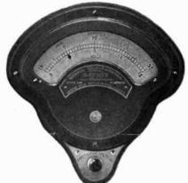
THIS Model normally indicates amperes, but upon pressing the contact button the pointer indicates volts so long as the button is held down.
