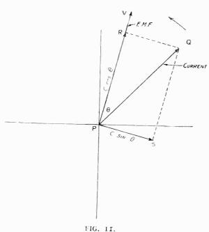
Therefore, as current  $C \sin \lambda$  (PS) does no work, it is known as the **idle component** or the **wattless component**.
