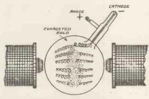
Fig. 5.—The Behaviour of Cathode Rays or Electrons when projected obliquely into a Magnetic Field.
