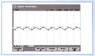
Figure 6: Output voltage ripple of the LTC3728 inverting buck/boost supply. V<sub>IN</sub> = +12V, I<sub>OUT</sub> = 15A
