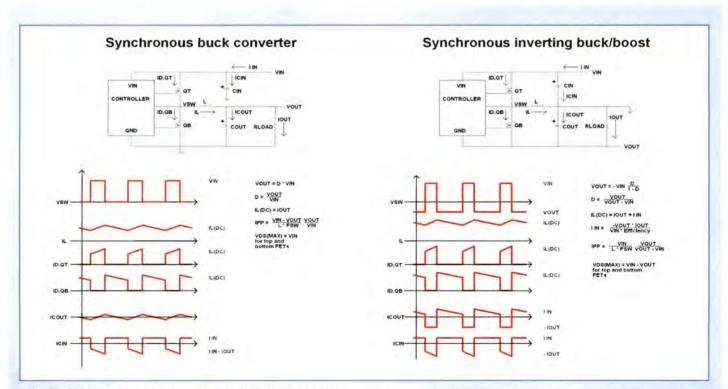
Figure 4: Comparison of a buck versus an inverting buck/boost
