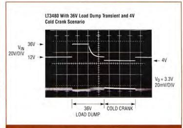
Figure 1: 36V load dump condition and cold crank conditions
