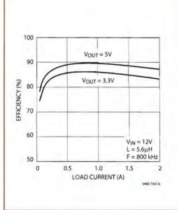
Figure 3b: The efficiency graph of the IC in Figure 3a
