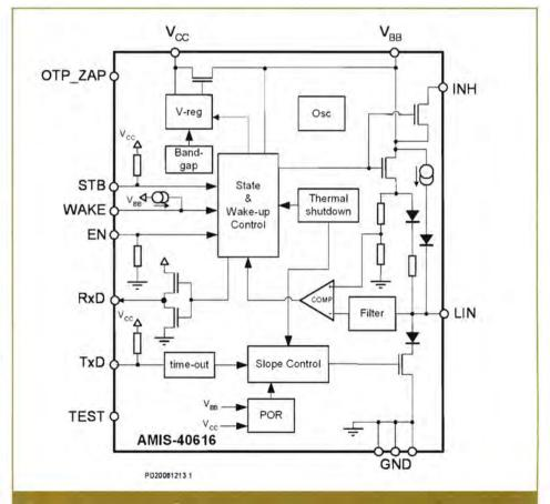
Figure 1: Block diagram of LIN transceiver IVN
