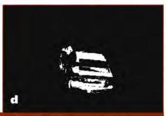
Figure 2: The current frame (a), previous frame (b), resulting difference image (c), binary image (d), obtained by thresholding the difference frame
