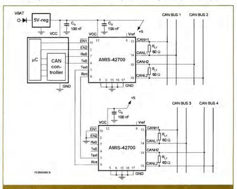
Figure 5: CAN repeater used as bus extender
