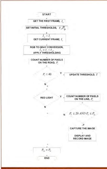
Figure 3: Flowchart of the detection software
