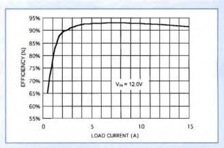
Figure 7: Efficiency of the LTC3728 inverting buck/boost supply
