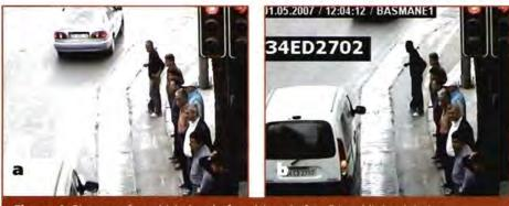
**Figure 4:** Pictures of a vehicle just before (a) and after (b) red light violation (red light violation system in Basmane-Izmir, Turkey)
