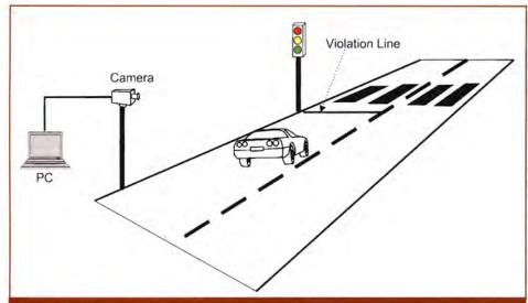
Figure 1: Red light violation detection system setup
