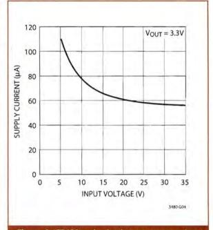
Figure 4: LT3480 no-load guiescent current vs input voltage
