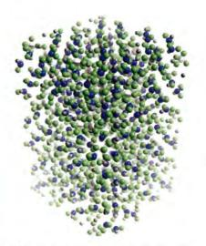
The future in store: hydrogen atoms can be absorbed effectively into the new storage material. Hydrogen (H) atoms are shown in green, lithium (Li) atoms in dark grey, nitrogen (N) atoms in blue and boron (B) atoms are in grey and inside the pyramids
