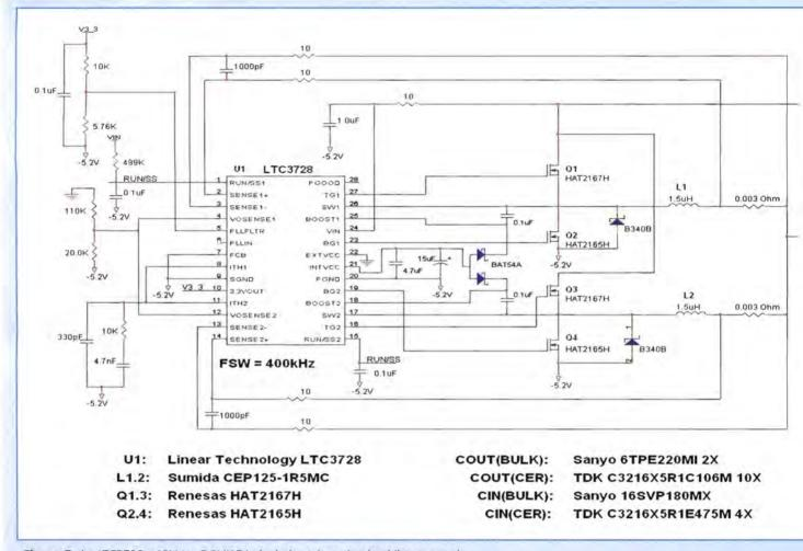
Figure 5: An LTC3728 +12V to -5.2V/15A dual phase inverting buck/boost supply
