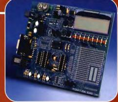
footprint, 2 x 16 liquid crystal display, PCB footprints for an H-Bridge motor driver, LIN transceiver, and a connector for programming via In-Circuit Serial Programming technology and developing with the MPLAB ICD 2 in-circuit debugger.
