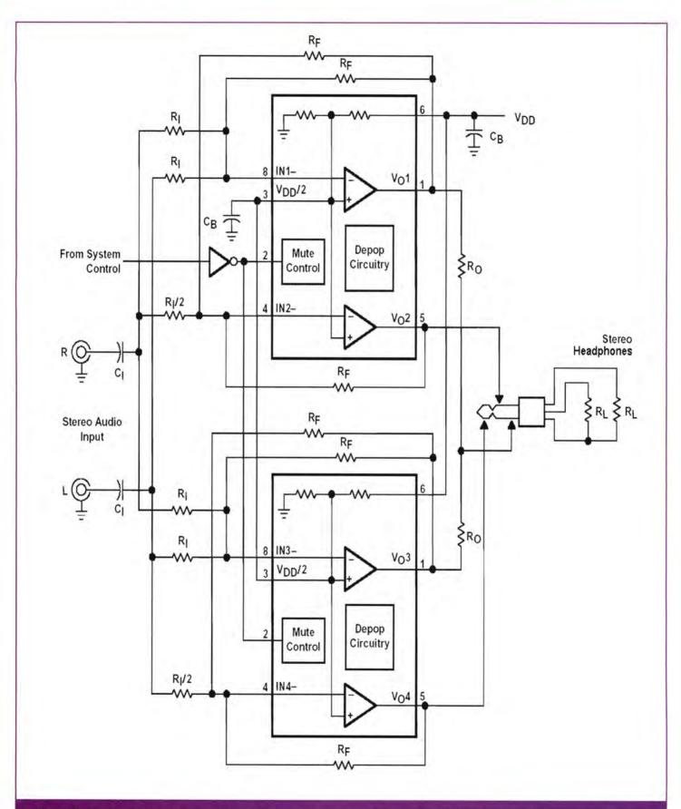
Figure 1: Two headphones chips and a handful of passive parts drive DC-coupled stereo headphones with common wire from the bridge circuit
