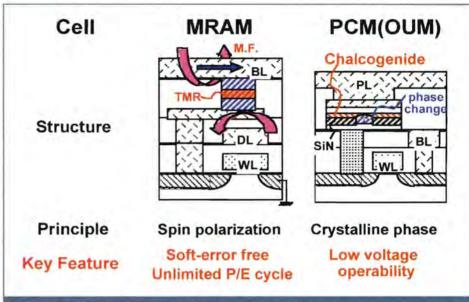
**Figure 4:** Next generation non-volatile memory technology. Magneto resistive RAM (MRAM) and phase change memory (PCM)
