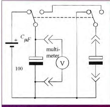
Figure 1: Capacitence meter
