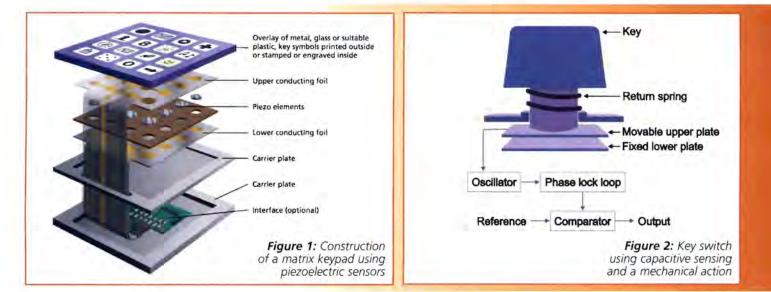
and 5N. The pills used in piezoelectric keyboards are typical around 200 microns thick and generate about 1VDC with an applied force of 1N. Within the last few years piezoelectric inks have replaced the pills in some designs, primarily to reduce assembly costs, but at the expense of an increase in applied pressure needed to produce sufficient voltage so that a switching action can be detected.
