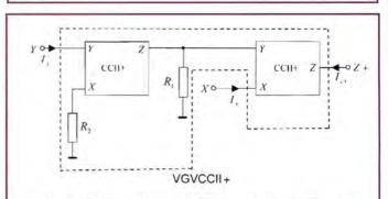
Figure 10: Realisation of a VGVCCII+ using two CCII+s and two resistors
