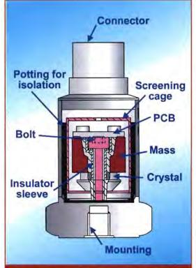
Figure 1: The mass (for a typical sensor) is bonded to a piezoelectric crystal which, when placed under tension or compression, generates an electric charge proportional to the acceleration of the mass
