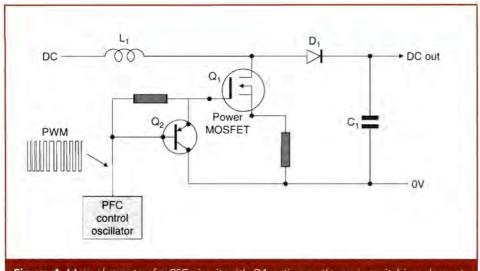
Figure 4: Main elements of a PFC circuit with Q1 acting as the main switching element
