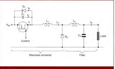
Figure 9: Zero Voltage Switching (ZVS) resonant converter
