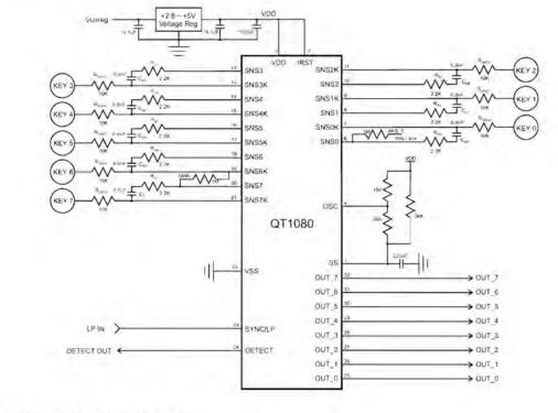
Figure 3: Example application of a matrix keyboard using charge-transfer sensing
