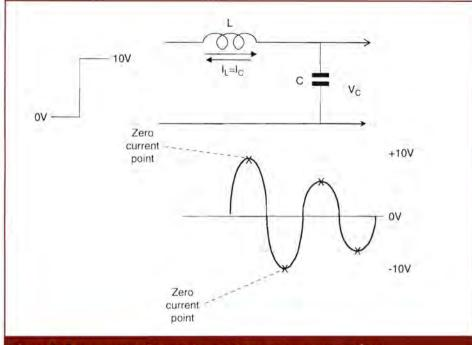
Figure 6: Zero-current and zero-voltage points on a resonant waveform
