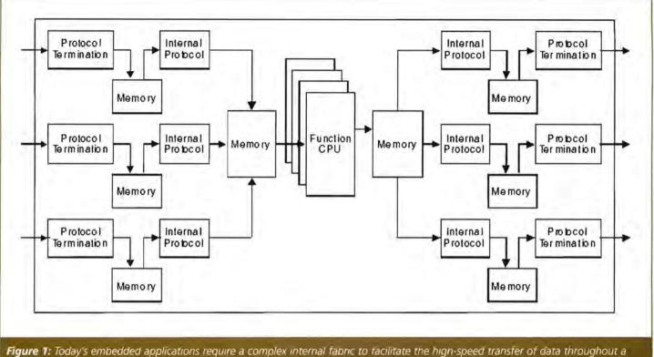
system, often passing through many interconnect layers and protocols, with each layer of interconnect introducing undesirable latency, complexity and cost
