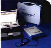
I GS/s sampling rate 250MHz bandwidth I28M sample buffer memory
