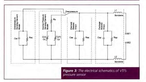
calculated as presented before. When the input pressure exceeds the normal mode, the output behaves according to overpressure sensing element model. In the element this means that the diagram touches the capacitor plate and the output is no longer a function of pressure. After the pressure comes back to the measuring range it again works according to the normal pressure sensing model with as good a performance
