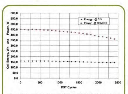
Figure 5: Energy and power evolution of Saft "VL45E" cells during cycling at 80% DOD DST cycle. Every 50 cycles, energy measured at 100% DOD – C/3, power measured at 80% DOD, 300A – 5mm pulse
