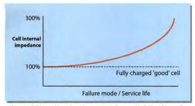
Figure 1 Cell internal impedance is not necessarily a good indicator of impending failure. It is not easy to detect the early stages of failure by this method
