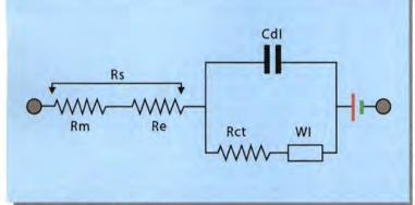
Figure 2: The Randles equivalent circuit for an electrochemical cell
