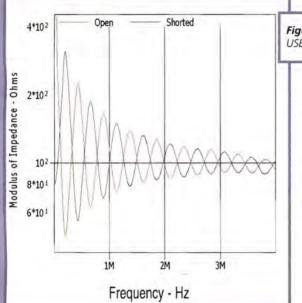
Figure 7: Response of a USB cable impedance
