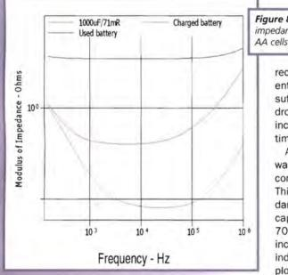
Figure 8: Battery impedance; two Ni-MH AA cells
