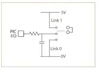
depending on the I/O output voltage allowing the "not connected" state. Software should check the "not connected" state first by driving I/O high, reading 1 and driving I/O low and reading 0. The "Link 1" and "Link 0" states are read directly.
