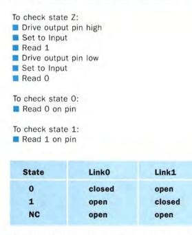
Jumper has three possible states: not connected, link 1 and link 0. The capacitor will charge and discharge
