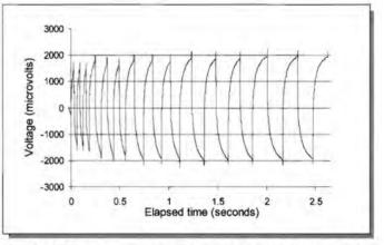
Figure 4d: Voltage response with the underlying micro-discharge 'drift' removed
