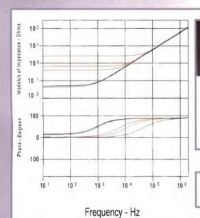
magnetic field strength and, also, their minimum useful operating frequency. The graph in **Figure 12a** shows a large spread in performance. One device only starts to behave as an inductor at 100kHz.
