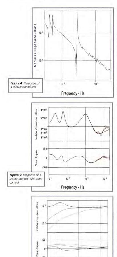
variation above 4kHz. The phase response in Figure 5 shows a ±45° variation, which presents a power amplifier with a reactive load that, at times, is half inductive or capacitive.
