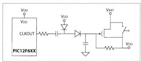
supplied to VDD and the MCU's CLKOUT (in external RC oscillator mode) begins to toggle. The voltage generated by the charge pump turns on the FET, allowing VDD to remain powered. To power down the MCU, execute a SLEEP instruction. This allows the MCU to switch off its power source via software.
