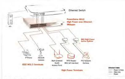
The High Power over Ethernet Midspan delivers up to 39W power over standard Ethernet infrastructure upcoming MIMO standard) and pan-tilt-zoom IP cameras. All these applications require typically more than 13W, normally between 13W and 30W. Going forward, laptops and even desktops could be powered too.
