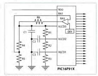
Figure 1: Voltage generator with resistor divider
