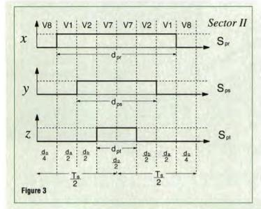
will be used in the present note, is shown in **Figure 3** for sector II. These signals can be applied for the remaining sectors by defining three auxiliary signals named x, y, z which are differently distributed to the transistor gates according to **Table 1**.
