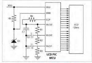
Figure 4: Software-controlled voltage generator
