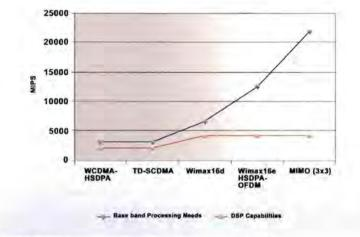
Figure 1: MIPS requirements for different wireless protocols
