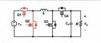
High efficiency non-inverting buck-boost DC/DC converter
