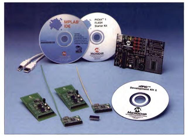
Lectronics World is offering its readers the chance to win a Microchip rfPIC Development Kit. The kit provides an easy way to evaluate low-power RF communication links for embedded control applications. Designed to work in tandem with the PICkit 1 Flash Starter Kit, the rfPIC Development Kit 1 includes transmitter and receiver modules supporting frequencies of 315MHz and 433MHz.
