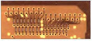
Grey items are printed OhmegaPly resistors on an IC. Longer ones at left are approximately 3 squares length; shorter ones at right are approximately 1 square
