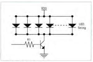
Figure 6: LEDs in parallel
