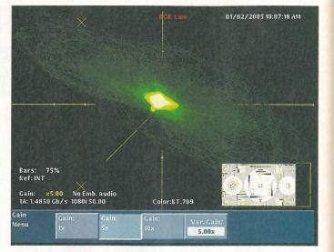
Figure 4: Magnified view of vectors cope display, showing a correctly white-balanced camera.
