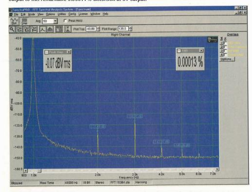
Fig. 10. This 20 year old 0.25 watt carbon film resistor made with a ground, not laser trimmed, spiral, produced 0.00013% distortion when loaded to 25% rated power. The second harmonic for a same make 0.5 watt resistor loaded to 12.5% rated power, measured 2.3dB better. Distortions from a modern laser spiralled, low cost 1% 0.5 watt metal film resistor, were too small to be measured.
