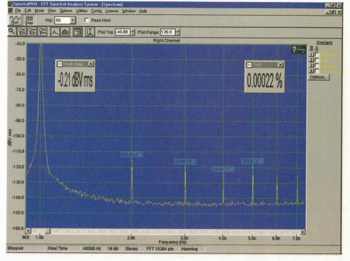
Fig. 7. Retesting the Figure 5 NE5532AN in the 'dual' amplifier test circuit as Figure 6, distortion has reduced again to 0.00022%, 50% less than the best 'single' amplifier of those tested
