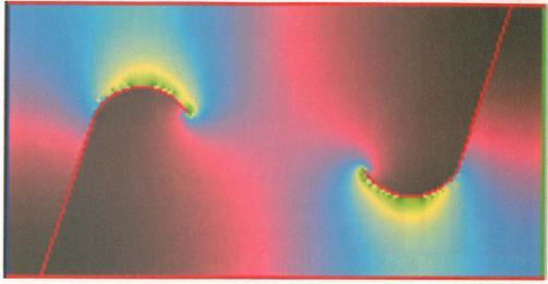
film is completely cut away. Thus the resistive material which has been overheated around the edge of the cut is no longer used to carry current.
