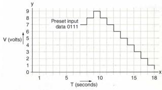
By loading the counter with preset data, the ramp can be made to start at any voltage.
