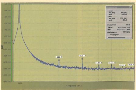
Fig 13. The Dr Jordan software, measuring a  $511\Omega$  resistor at 1V and 1kHz.
