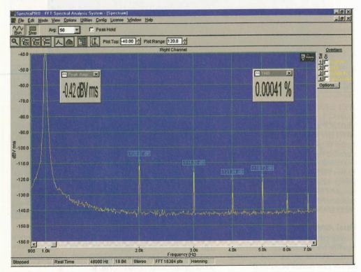
Fig. 6. The TL072CP of Figure 4, tested in the 'dual' amplifier circuit using its 'A' half for gain and 'B' half as a voltage follower driving the test load. Distortion has dramatically reduced from 0.01266% to 0.00041%.
