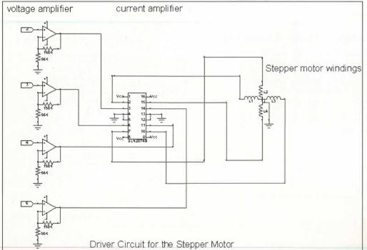
In the circuit shown below a 12V, 1.5A, 10kg - cm torque stepper motor is interfaced to the PC via its parallel port. This is done in order to automate the motion of the stepper motor. This circuit is mainly IC based which makes it easy for construction. has fewer components and is also cost effective.
