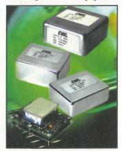
The device is designed to provide a holdover performance of better than  $7\mu s$  over 24 hours in stable ambient conditions and a frequency stability better than  $2 \times 10^{-10}$  peak-to-peak over an operating temperature range from -20 to  $+70^{\circ}$ C. Package size is  $51.0 \times 41.0 \times 19.0$ mm. C-MAC Micro Technology www.cmac.com
