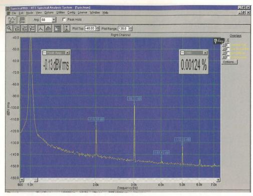
Fig. 12. Re-connected as potentiometers to output a 3V test signal drawing 225µA through their wipers, produced a similar pattern of distortion. The cermet control with 0.00124% distortion was worst; the low cost carbon was much better at 0.00039%, the conductive plastic and wirewound measuring just 0.00009% and 0.00005% respectively.
