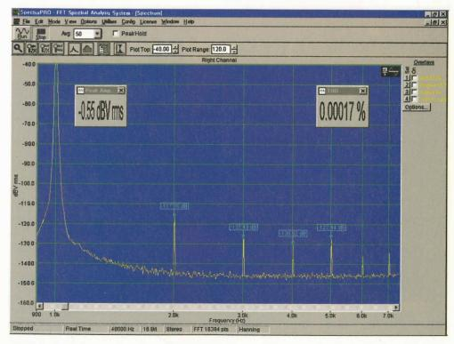
Fig. 8. Removing the DIL header and R28 to use two separate ICs rather than the 'dual' arrangement of Figures 6 & 7. Retesting the Figure 5 NE5532AN 'A' section with an NE5534AN for U8 removed the test load thermal effects, reducing distortion to just 0.00017%, halving that measured with the best performing 'single' IC
