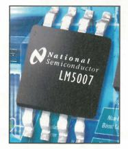
0.7A peak that can be switched at high frequencies (up to 500kHz), allowing the use of a small output filter to complete a bias supply design that sources up to 0.5A continuous load current. The device is available in a 4 x 4mm 8-pin chip-scale package and an MSOP-8 package. According to the supplier, the control scheme
