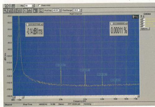
Fig. 9. Refitting R28 and using an AD811AN current feedback amplifier for U8, this Burr Brown OPA2134CPA, the joint best 'single' amplifier tested, reduced its distortion from 0.00036% at 4V output to this remarkable 0.00011% distortion at 6V output.
