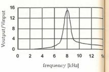
Fig.3. Frequency response of the oscillatory circuit.
