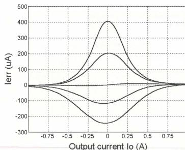
Due to closely matched transconductances (within 5%) and high Early voltage (over 300V) for both N- and P-channel parts, the results were far better. The error function, **Fig. 6**, is in accordance with the simulation, although skew is slightly higher and in the opposite direction. Ripple currents were hardly measurable.
