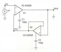
Fig. 2. The schematic from the "Active Feedback Amplifier Enables High-Performance A-to-D Conversion" article<sup>2</sup> found while accessing the Electronic Design web
