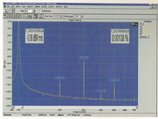
Fig. 11. This multi-turn cermet trimmer, set as a  $5.6k\Omega$  variable resistor and tested with a 6V signal from  $1k\Omega$  source impedance, generated this enormous -97dB third harmonic, 0.00138% harmonic distortion. Tested exactly the same a low cost carbon control produced 0.00129% while a conductive plastic control and 10-turn wirewound generated only 0.00009% and 0.00007%.
