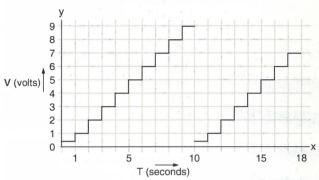
Output waveform when the circuit is used as a staircase generator.
