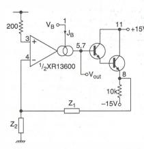
Using a transconductance op-amp, one simple circuit can act as a voltage-controlled resistance, capacitance or inductance.
