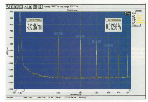
JFET input TLE2072CP measured 0.00142%, much better than the old TL072CP and slightly better than the AD712JN while an OP275G with its Butler Bi-polar/JFET input stage, intended for audio circuits, measured 0.00088% distortion. The Burr Brown FET input OPA2134CPA, part of their 'SoundPlus' range designed for low distortion audio, measured 0.00036% to equal the NE5532AN performance. Fig. 5.
