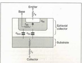
Fig. 4. Diagram of bipolar transistor showing model parameters. Total base-emitter capacitance is  $c_{bt}$  while  $r_c$  and  $r_e$  are shown partly outside the device to represent contact resistance from the metal to the semiconductor.
