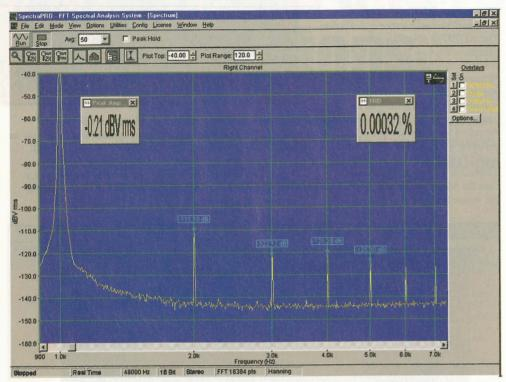
Fig. 5. Tested at 4V output, but otherwise exactly as Figure 4, this 'single' amplifier test of an NE5532AN produced remarkably little distortion driving this difficult test load, a heavier load than would be expected in any real world circuit or interconnect cable loading.
