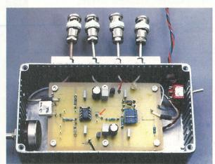
Fig. 1. This test PCB, attached to my real-time hardware distortion analyser, was used for more than 75 distortion measurements of the IC op-amps and test circuits in this article, simply by unplugging ICs. Switching the link shown arrowed, changes from the 'dual' amplifier position shown to 'single' using the 'A' section only of the IC. Replacing the DIL header with an IC, changes from measuring U7 to the two amplifier circuit, U7 and U8.
