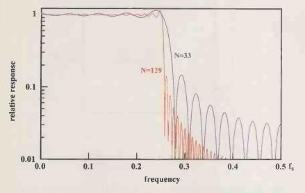
Figure 4. Frequency responses of lowpass filters of lengths 33 and 129. informal cut-and-try approach is usually surprisingly fast. The only changes that are made in each iteration, other than to the original filter specification, are to filter length and to the window function.
