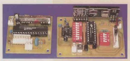
that are suitable for extended range data link at a data rate up to 10kb/s<sup>1</sup>. A range of 10km can be achieved in open ground with a suitable data rate and antennae. They are typeapproved to the EN300 220-1 for use at 173.250MHz in the UK and fully screened with extensive internal filtering to ensure EMC compliance to ETS 300 683. Other frequencies are available from the manufacture<sup>1</sup>.
