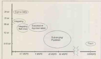
Fig. 5. Map of A-to-D conversion resolution against conversion rate for the main technologies in use today.
