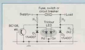
Under normal conditions, this monitor circuit indicates the powered-up state via green light from a three-colour LED. If the fuse blows, the LED turns red.
