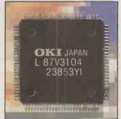
16/256 colours out of 4,096 colours (pseudo colours) and 4,096/6,5536 (direct colours). Output data complies with STN 4/8-bits parallel or TFT 12-bits (R4, G4, B4) or 16-bits (R5, G6, B5). An extended temperature version is available (-45 to 85°C). Oki Electric Tel: +44(0) 1753 787700 www.oki-europe.com
