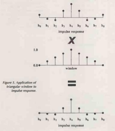
from the Fourier transform of a response specification that has a discontinuity and we were forced to truncate the impulse response to a finite length, in this case 33 or 129 (that is, we calculated only 33 or 129 values of the infinite series).
