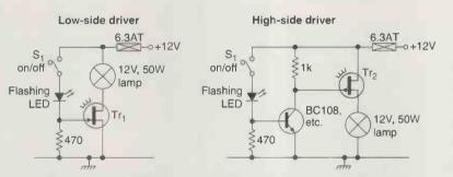
The second circuit is the high-side driver. Again around 6 volts is developed across  $R_1$  when the LED is on. Voltage across  $R_1$  does not go sufficiently low to turn on the MOSFET when the LED is off so a simple inverter is introduced to enable the MOSFET to be fully turned on.
