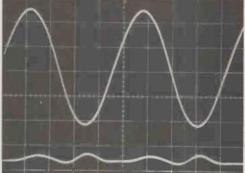
Photo 4 Waveform resulting from driving the amplifier at 40W,  $8\Omega$  with a 100kHz sine-wave illustrates the absence of switching distortion.
