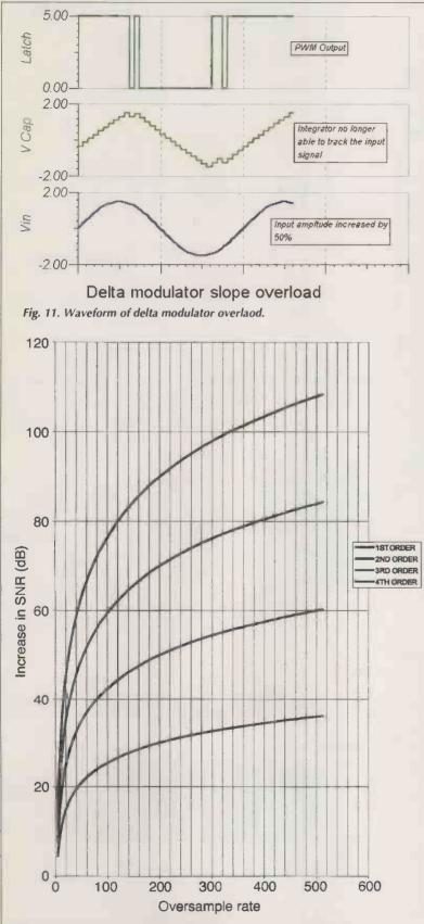
Fig. 12. Plot of signal-to-noise ratio improvement versus sample rate and modulator order.
