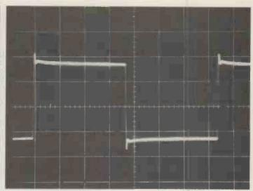
Photo 2 Square-wave response (2kHz) at RL=8Ω
