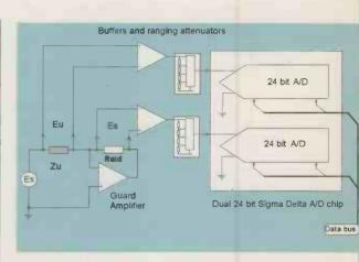
Fig. 13. Elements of a simplified LCR bridge based on DSP.
