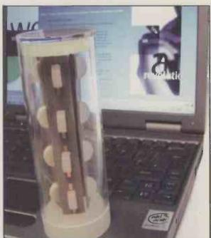
A five-sectored array for 5.8GHz wireless LAN infrastructure. The 72° sectors allow spatial diversity to increase in-room data rate. Four elements per sector produce a 20° vertical beam to increase gain. The array can also be set to omnidirectional mode.
