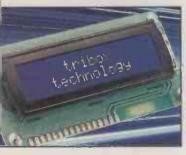
design assistance and programming should this be required. The displays use STN glass with white LED backlighting. In reverse mode blue on white is also possible. *Tribox*
