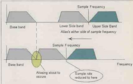
Fig. 1. Aliasing occurs when the sample rate is reduced below twice the base-band maximum frequency.
