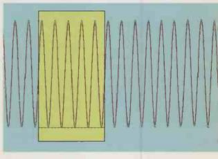
Fig. 14. By sampling from zero crossings and whole multiple periods of the measured signal, perfect windowing is obtained by the FFT. This avoids spectral leakage or blurring of the FFT output spectrum.
