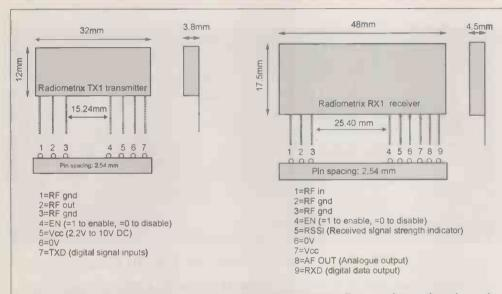
TX1 and RX1 are a licence-exempt miniature 173.250MHz VHF radio transmitter and receiver pair suitable for long-range data links. Link range of 10km is achievable with choice of data rate and antenna. They are completely screened with internal filtering to meet EMC requirements. Other frequency versions are available from the manufacturer. examples. Range tests should be performed to establish the actual link range.
