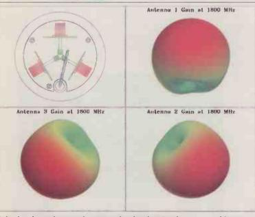
Gain plots for a tri-sectored antenna, showing the 3D gain pattern - with pattern length and deeper colour indicating higher intensity
