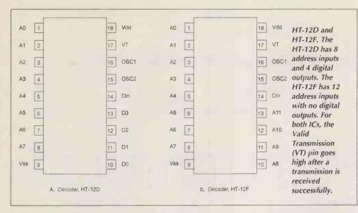
both ICs, the VT pin (Valid Transmission) goes high after a valid transmission is received. An oscillation resistor shall be chosen to suit the frequency of the signal produced by the encoder (**Ref 3**).
