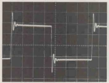
Photo 3 Square wave response (2kHz) at CL=1µF
