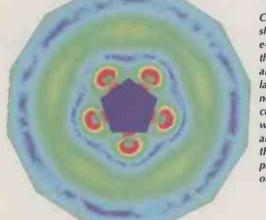
Computer simulation shows a top view of e-field intensity from the 5-sectored router antenna shown in the laptop picture. The near field is almost completely contained within the dielectric antenna elements and the far field propagates omnidirectionally.
