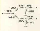
Fig. 5. The splitter and 3dB pads are ideally as shown. In practice, they will consist of standard value resistors as in Fig. 4.
