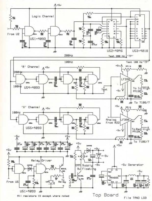
Fig. 2a) Complete schematic, including all supply line decoupling, for the right hand or 'Bottom' board, shown in Fig. 1. Fig. 2b) is the complete schematic, including the floating 9V supply for the PM128 display, the -5V converter and all supply line decoupling, for the left hand or 'top' board in Fig. 1.
