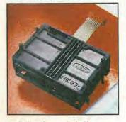
product can be supplied with a standard stack height or with a raised floor that lets components be mounted on the PCB beneath the connector. It is possible to use a variable thickness connector as the lower part. The connector is assembled using clip-on techniques and the module's spring contacts. AMF
