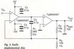
implemented, this deceptively simple circuit produces a 1GHz gain bandwidth product. With values shown, gain is 40dB with a -3dB response of 10MHz. The circuit can drive up to ±3.3 volts into a back terminated  $75\Omega$ coaxial cable.
