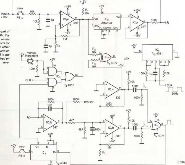
arrangement senses polarity, corrects for a zero voltage offset and produces an output equal to the input, but centred on
