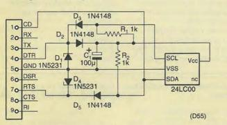
In devices needing electrically readable serial numbers, the 24LC00 16-byte eeprom is tiny and provides a 32-bit number. The circuit shown programs the eeprom from a pc's serial port.
