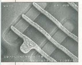
Tiny tracks... Getting to 0.13µm features using existing 248nm lithography has resulted in the use of phase shift masks and other complex techniques. IMEC's work on 193nm processing will enable 0.13µm and 0.10µm without these expensive add-ons.
