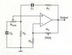
Fig. 3. A modification permitting ±9% tuning range, with negligible effect on output level.
