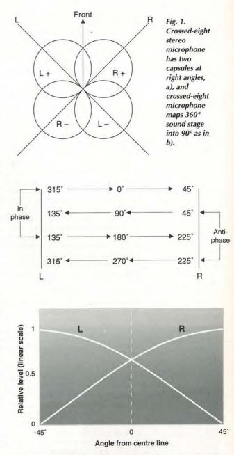
Fig. 2. Apparent position of the virtual sound source is a function of the level difference between the channels. This defines the characteristics that a microphone must have.
