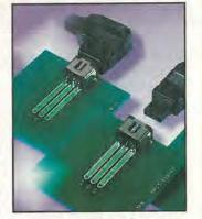
up to 5A, 30V AC and 42V DC. The connector can be fully polarised with two or three contacts, with the three pin version having one leading contact for grounding. The PCB mounted parts are 7mm deep with a metal cover that provides a snap lock mechanism. The two-way plug comes as a prepared cable assembly with straight cable exit. The three-way is available in straight or right angled versions and is wired using crimp contacts and snap together hoods. Hirose Tel: 01908 260616
