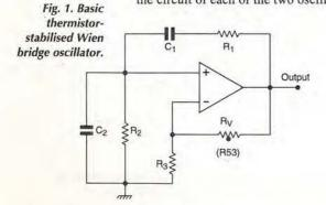
tors he used. Each could be set for one of two pre-set frequencies – switching arrangements not shown here – the output level being stabilised as usual with an R53 thermistor.
