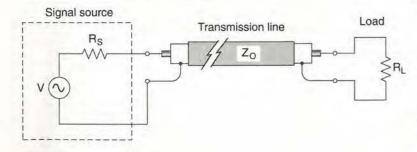
Fig. 2. Since it is not usually possible to site a transmitter right next to its load, power is normally passed to the load via a transmission line with a characteristic impedance, Z<sub>0</sub>.
