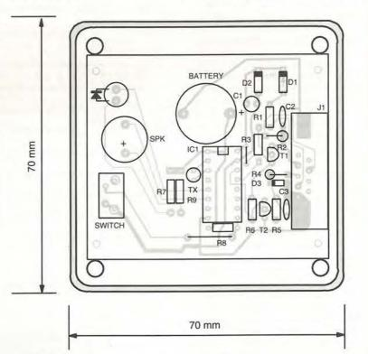
Fig. 7. The single-chip temperature logger can be constructed on a single-sided board and housed in a vented box. This figure shows the component layout of the PCB.
