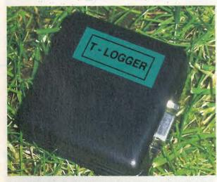
Fig. 1. Temperature logging is made simple - and small - using a sensor with integral digitising, control and serial i/o.
