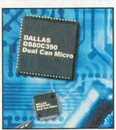
memory and 4Mbyte of external program memory. Applications include factory automation, marine control and navigation, industrial control systems, and HVAC control. *Dallas Semiconductor Tel: 001 972 371 3832* Enquiry No 521
