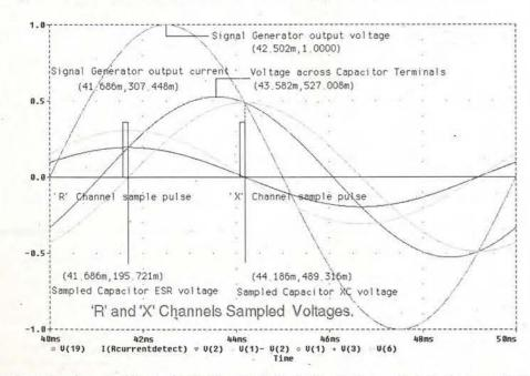
Fig. 5. Sample-and-hold control pulses from the logic circuit, superimposed onto the test capacitor's current and voltage waveforms. The phase angle between the capacitor current and the voltage developed across its reactance remains precisely at 90°, or 2.5ms, at 100Hz. The meter design relies on this relationship.
