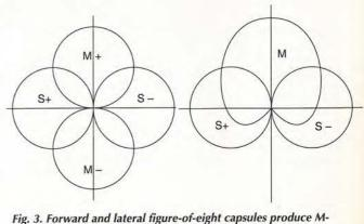
adding and subtracting proportions of these four signals in various ways it is possible to synthesise a stereo microphone having any acceptance angle and to point it in any direction relative to the body of the microphone. This can be done using the control box supplied with the microphone.
