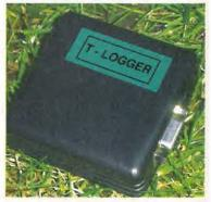
Small, simple and battery operated, this temperature logger wakes up from time to time to take a reading. When it's full, it connects to a PC for data uploading. See page 26.
