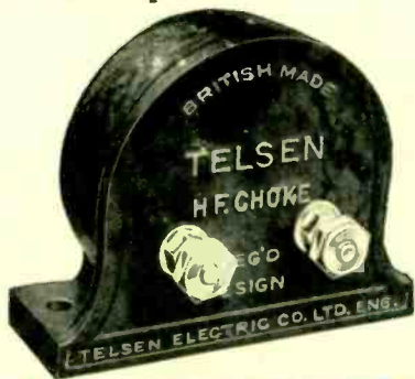
TELSEN H.F. CHOKES designed to cover the whole wave-band range—from 18 to 4,000 metres, extremely low self-capacity. Inductance 150,000 microhenries; resistance 100 ohms. Price 2/6 each.
