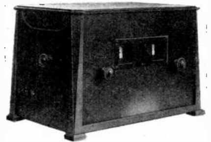
The new G.E.C., 3-valve all-mains receiver, housed in a cabinet of striking design, and priced at £18.
