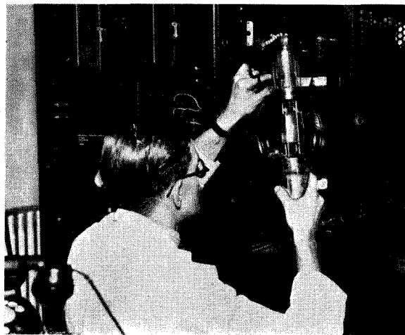
Valves for special purposes are often very much bigger than those to which we are accustomed in radio reception. The example seen here is a high-power amplifying valve used by H.M.V. for gramophone recording
