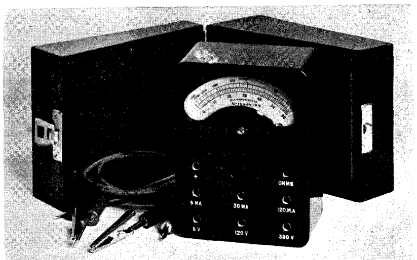
One of the handiest—and cheapest—of testing instruments is the Avomitor. It is a combination meter which gives measurements in ohms, volts, and milliamperes: the actual ranges are given in the article
