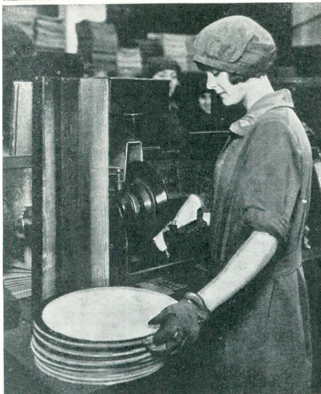
Columbia photo Fig. 6.—Here the operator is seen buffing, or trimming, the rough edge of the record as it revolves rapidly in a special machine. First of all a coarse abrasive paper is used. This is followed by a fine grade and lastly a polishing pad completes the process. Cardboard discs are placed between the finished records to prevent them being scratched
