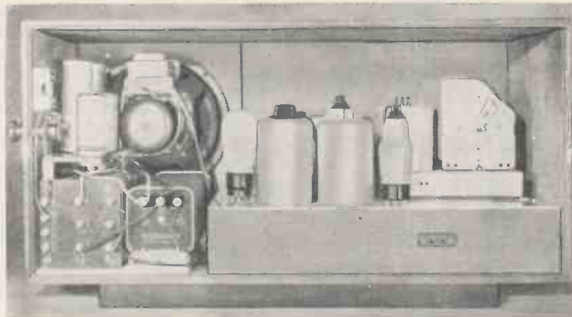
HOW THE SET FITS IN ITS CABINET Showing the A.C. Stenode in its cabinet. There is plenty of room. Note that the mains unit—on the left—has been built to fit round the energised moving-coil loud-speaker
