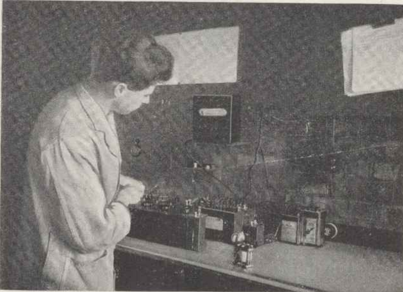
A corner of Paul Tyers' laboratory where the "W.M." Stenode receivers were designed. Here one of Mr. Tyers' assistants is measuring the permeability of alloy transformer stampings at 50 cycles under normal operating conditions
