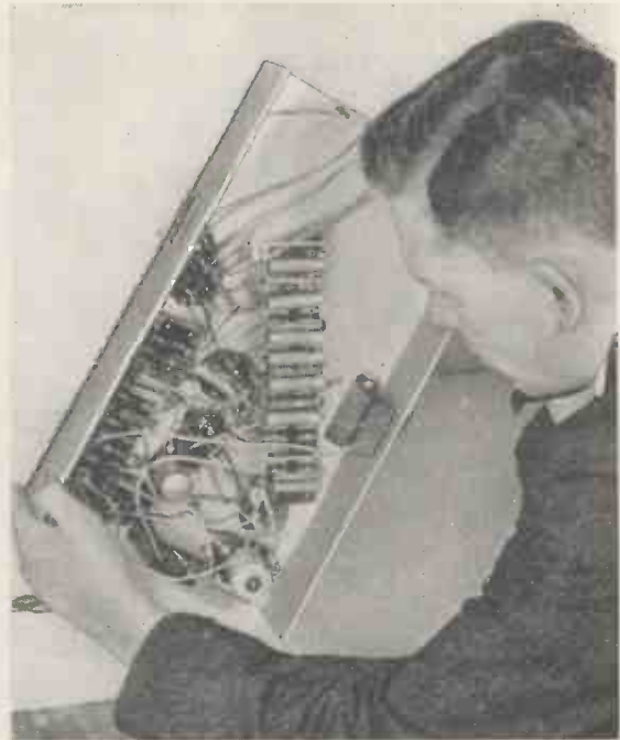
LOOKS ARE VERY DECEPTIVE! At first sight the underside of the battery Stenode appears to be a complicated business. Actually construction is very simple—all the resistances and condensers are mounted separately on sub-assemblies
