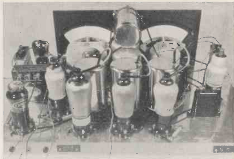
Owners of original Super 60 and Super Senior sets can use up many of their present components. The valves, from left to right, are class-B, driver, second detector, oscillator behind the two intermediate-frequency amplifiers, first detector and H.F. amplifier.
