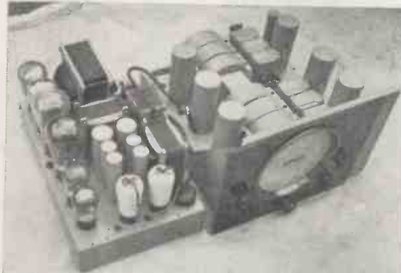
A 10-valve straight set for the connoisseur made by Hacker's of Maidenhead. Note the large tuning dial
