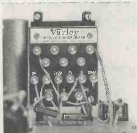
This photograph shows clearly how the various wires are taken to the terminal board of the mains transformer. The set is suitable for any A.C. mains voltage between 200 and 250
