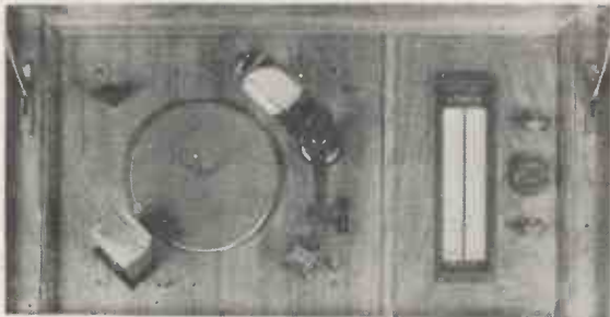
The motorboard of the H.M.V. model 580 autoradiogram. A neat layout with the visual tuner at the top of the tuning scale
