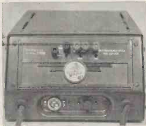
The panel of the Atlas A.C. mains unit showing the voltage tappings at the top and the trickle-charger switch below
