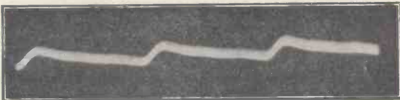
Fig. 6.—Mains current with poor smoothing following half-wave rectification; the ripples cause mains hum in the loud-speaker
