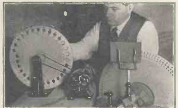
On the left is seen a scanning disc for 30-line pictures, and on the right a disc for 100-line pictures, which, of course, give greater definition.
