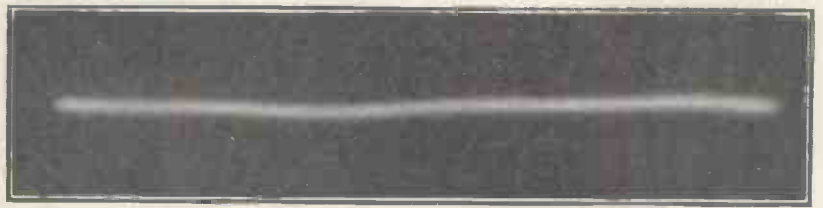
Fig. 8.—Oscillogram of properly smoothed mains supply. It is practically a straight line and there are no ripples to cause hum
