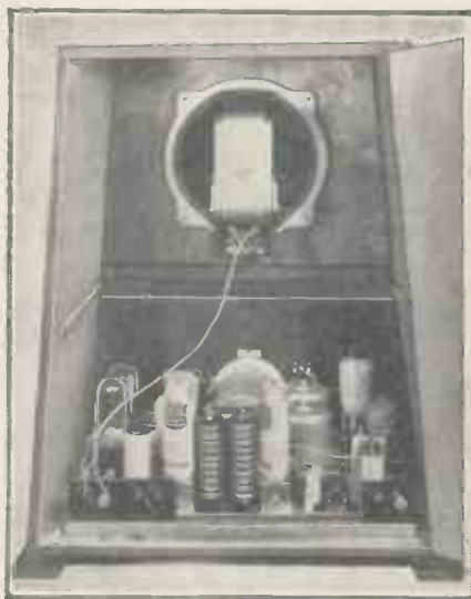
ALL READY FOR USE Here is the A.C.-D.C. Three assembled as a console table model with built-in moving-coil loud-speaker
