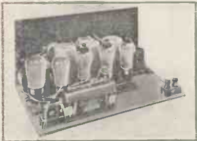
Designed by W. G. Hill. Circuit: 5-valve short-wave super-het. Price of set: £6 10s. without valves.
