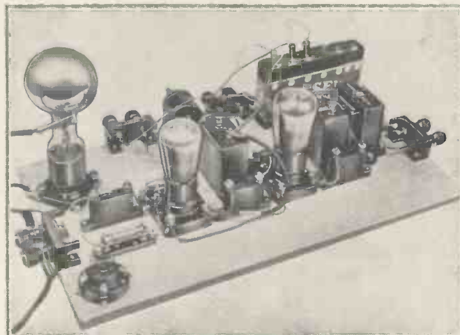
This photograph shows the amplifier suggested by Percy W. Harris for simple photoelectric experiments, which open up an entirely new field for the amateur
