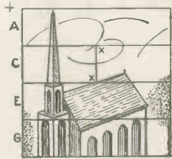
Fig. 1.—Picture divided into horizontal strips for analysis by the mirrors or prisms
