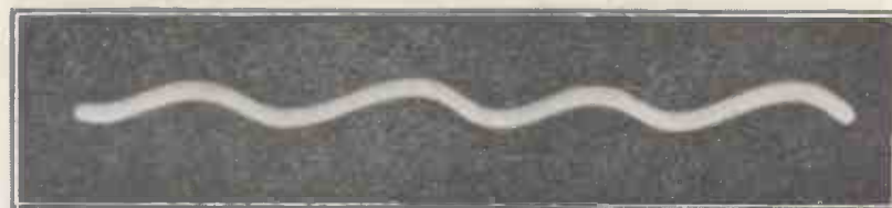
Fig. 7.—Another example of a poorly smoothed mains supply, which will also cause hum. This is from a full wave rectifier
