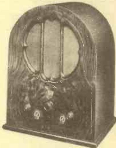
Cossar model 221 De Luxe, a battery two-valver. The loud-speaker adjustment is at the back
