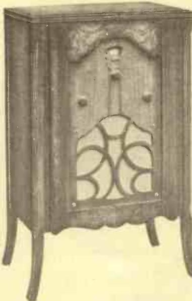
Alba model 66 for A.C. and D.C. mains, a three-valver with a moving-coil loud-speaker
