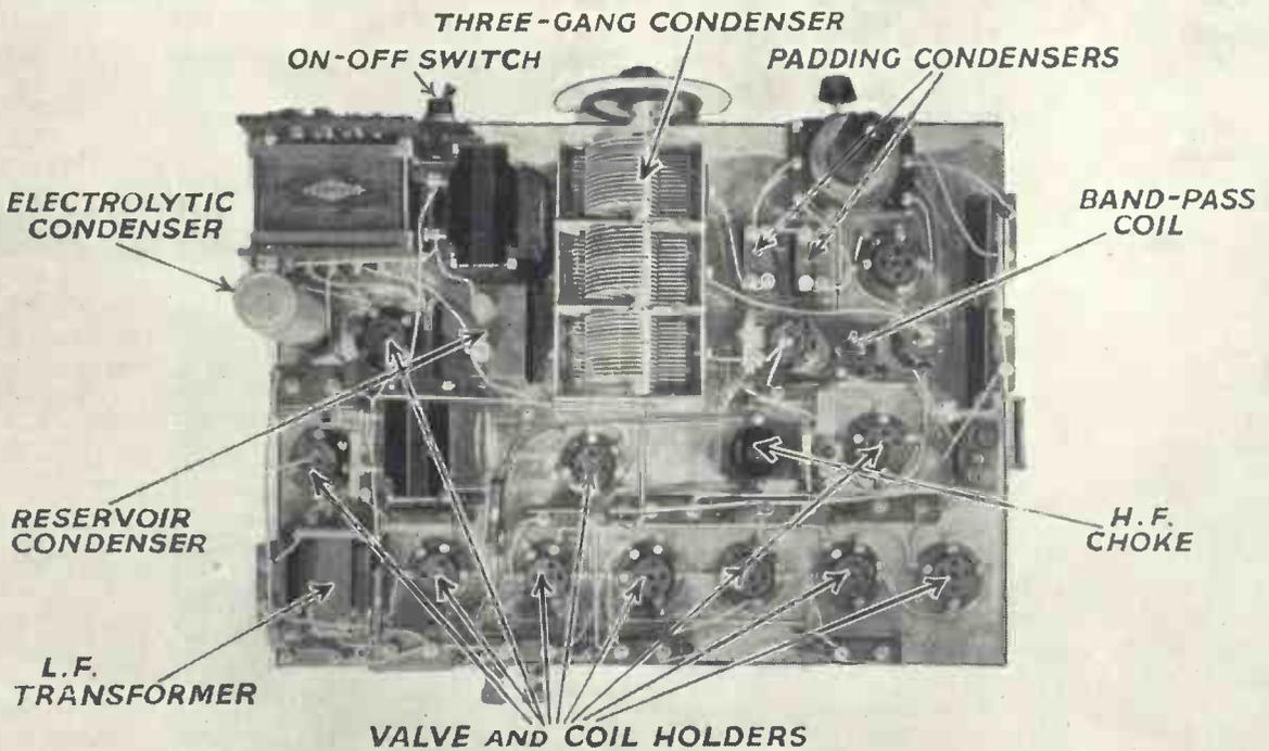
This photographic plan view of the Seventy-seven Super gives a clear indication of the arrangement and disposition of the components. A standard three-gang condenser is used
