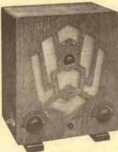
A two-valve battery set, type S328, made by Standard Telephones and Cables, Ltd.
