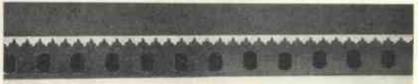
Fig. 3.—Organ pipe Middle C. The fundamental measures 257 c.p.s., which agrees closely with the theoretical 256 c.p.s. The second harmonic is seen to persist at about 60 per cent, with a very slight trace of third harmonic. This condition remains constant
