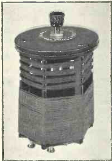
TYPICAL DUAL-RANGE WINDING In this coil the long-wave winding (seen at the top) is arranged in slots in the ebonite former
