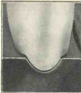
Fig. 3.—Loud needle after playing six 12-in. sides
