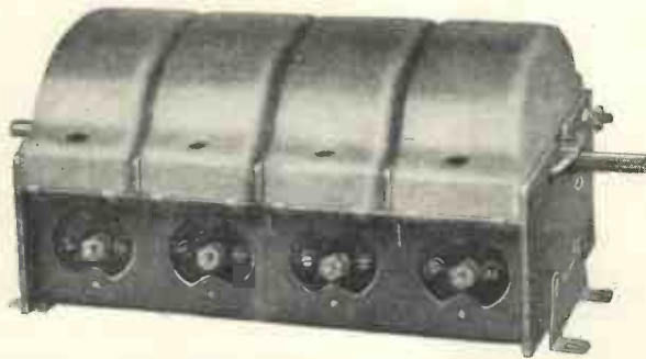
(Above).—A new four-gang condenser introduced by Polar this season, the Star model. The trimmers are fitted on the top
