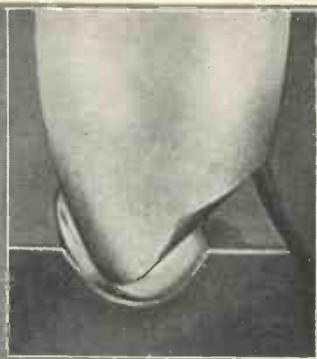
Fig. 4.—As in Fig. 3, but with needle skewed across the groove
