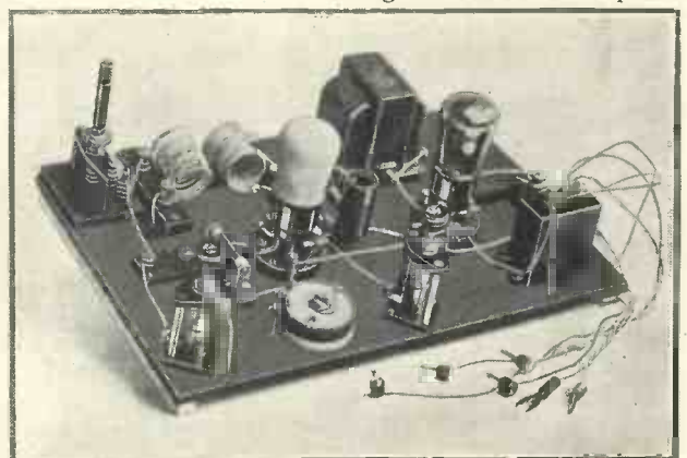
A NEW FIELD FOR THE KEEN FAN The new 7-metre transmissions open up a new field for the keen experimenter. This simple set can be built at very low cost
