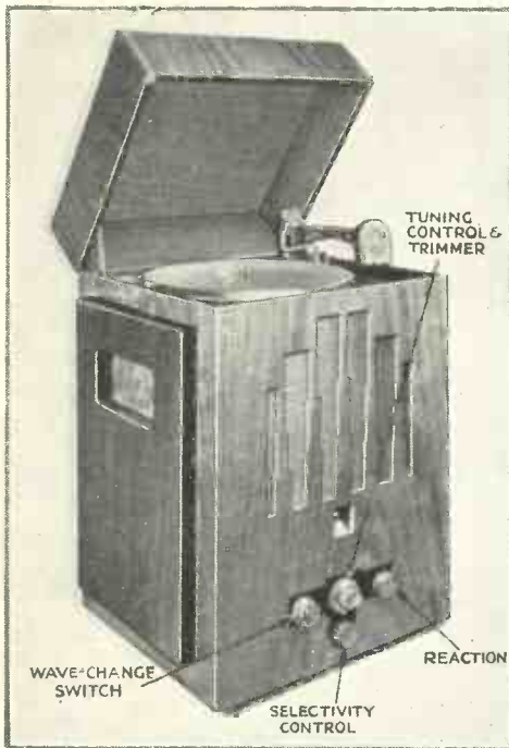
A COMPACT INSTRUMENT Except for the aerial and earth, the Climax tabl. radiogram is entirely self-contained
