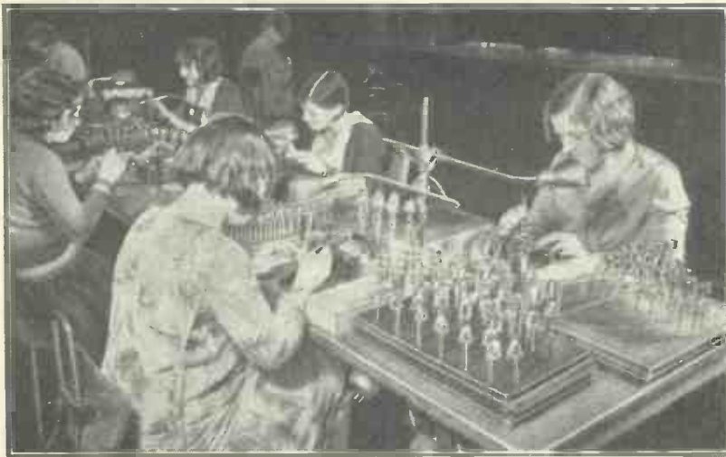
ASSEMBLING THE COMPLETE ELECTRODE SYSTEM Fig. 5.—Here the parts are skilfully assembled on the stems
