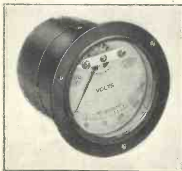
A high-resistance 0-250 moving-coil D.C. voltmeter made by Sifam. The resistance is 1,000 ohms per volt and the price is £2
