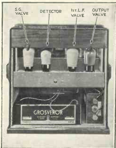
ACCESSIBLE COMPONENTS A photograph showing the set with the back removed. Batteries and valves can be easily changed
