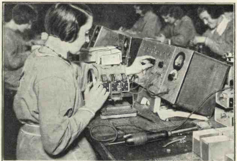
PRECISION TESTING TO ENSURE ACCURATE GANGING Testing and adjusting band-pass and super-het condensers in the Ferranti works at Hollinwood. Great accuracy is needed for efficient one-knob tuning
