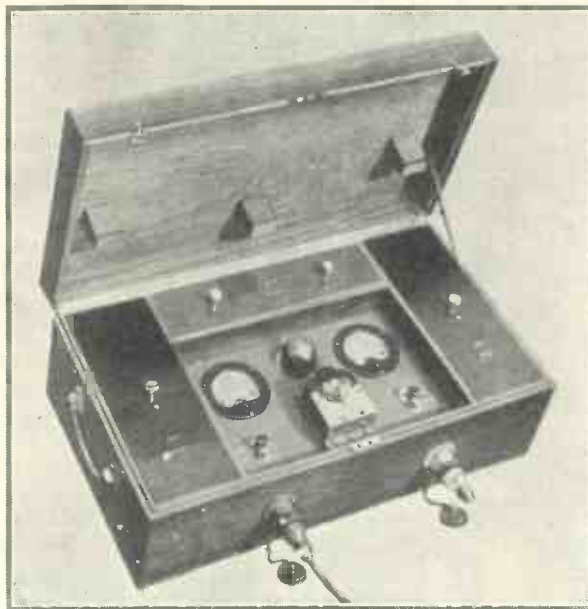
WORKED FROM THE ELECTRIC MAINS The Audiovisor bridge with relay and amplifier operated from the mains
