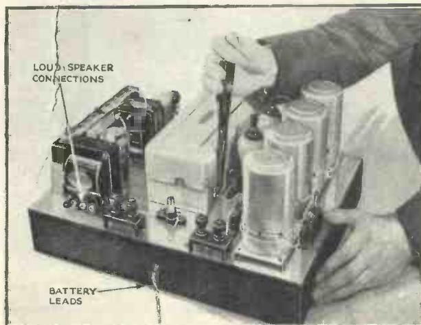
ADJUSTING THE TRIMMING CONDENSERS A pair of long-nose pliers will be needed for adjusting the screw heads of the four trimming condensers. The operation is not at all difficult
