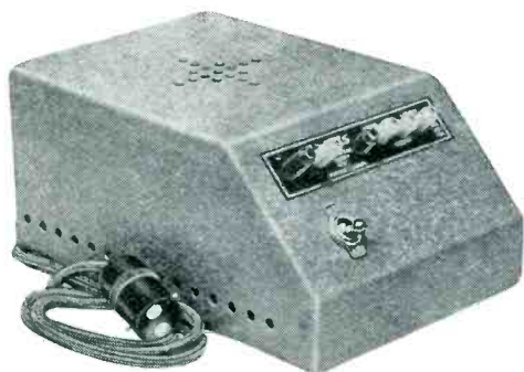
A new Atlas mains unit for high tension and trickle charging
