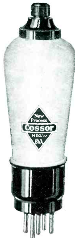
Metallised mains screen-grid valve—the Cossor MSG/HA
