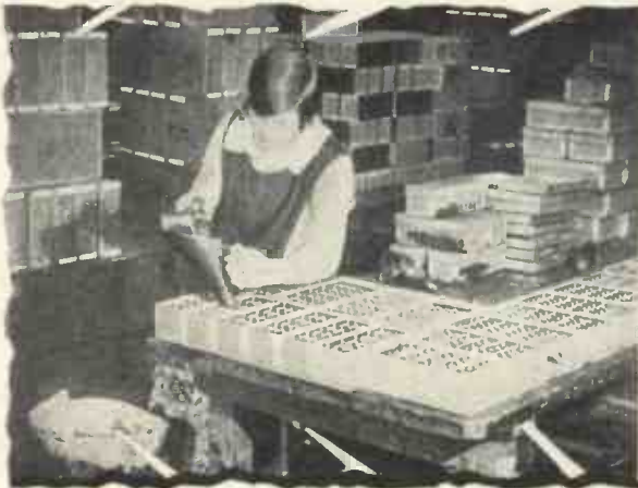
Filling Siemens battery containers with insulating wax
