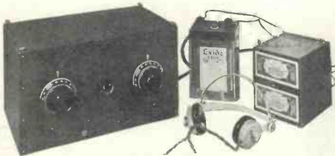
Gecophone short-wave three-valver connected up ready for use
