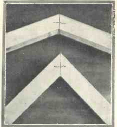
The framework is jointed by means of carpenter's "dogs"
