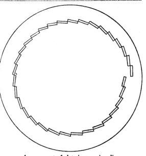
Arrangement of slots in scanning disc
