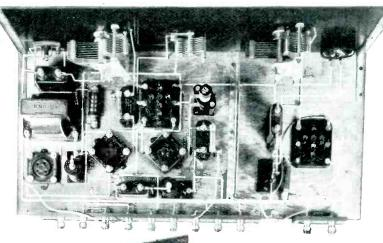
The above plan view of the Arrow Four clearly shows how all the parts are laid out; there is no overcr owding
