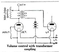
obtain satisfactory working when a volume control of this type is not fitted, for the stronger signals would tend to overload the detector. There are occasions, however, when a second regulator is necessary and, as an example, I will refer to a set having an anode-bend detector with one high-frequency and two low-frequency amplifiers that is also employed for playing gramophone records.
