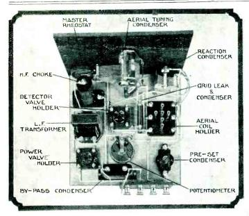
In other words, the lower the reading of the main tuning condenser less capacity is needed in the reaction condenser to put the set on the verge of oscillation; but as the main tuning condenser is put further into mesh it will be necessary to increase the setting of the reaction condenser.
