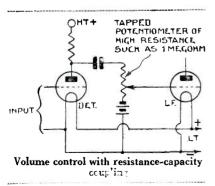
the valve, to which the pick-up is connected, is of a type that will take a grid bias of about 3 volts negative with normal high-tension. If the valve is of a type that will not stand a grid bias of more than negative 1.5 volts, there is a little danger should the pick-up be of the most sensitive type and be playing a loud record.
