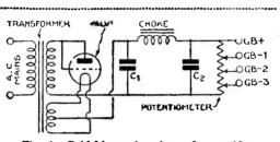
Fig. 4.-Grid-bias unit using valve rectifier
