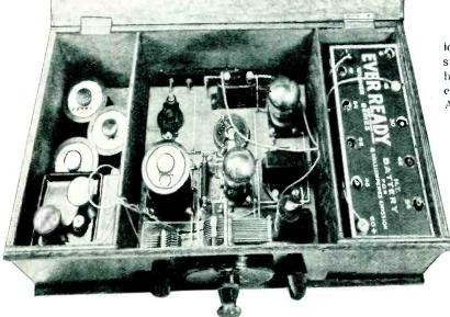
This photograph shows the batteries and spare coils in position in the special compartments provided for them
