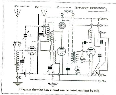
H.F. choke, and the other to H.T. + IThese four temporary connections are shown in dot-dash lines in the diagram.
