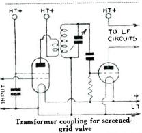
may, however, be made almost identical with that to be obtained from a suitably tapped anode coil. Theoretically, a tapped anode coil and a transformer give identical results, but in practice the transformer must be just a little inferior There is very little in it when the transformer is a good one. S.M.
