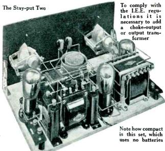
normal con struction. Α U5 valve is employed for rectifying the A.C. and a simple chokecondenser smoothing system is all that is required. It will be noticed that a 2-microfarad reservoir condenser and a 2-microfarad smoothing condenser are used. These capacities are smaller
