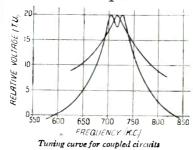
THE benefit of using two or more circuits in cascade, as suggested in Sheet No. 142, is that the tuning some distance away from the resonance point is sharpened considerably, whereas around the resonance point itself the twing hormes flatter.
