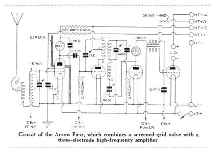
amplification which is not tuned, a stage of neutralised high-frequency amplification employing a threeelectrode valve, a leaky-grid detector, and a transformer-coupled low-frequency stage.
