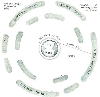
Diagram showing electron belt theory of wireless echoes. The wireless waves from the earth penetrate the Heaviside layer—strike the electron belt and are reflected back to earth
