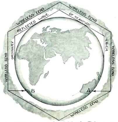
Diagram showing Heaviside layer theory of wireless echo. Wireless waves are radiated from the earth at A, travel round the world (thick line) about 100 times within the confines of the layer and, by some freak, return to the earth at B.
