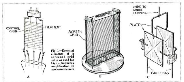
A ordinary receiving valve, but having a wire-mesh screen fitted must be properly connected to the circuit.
